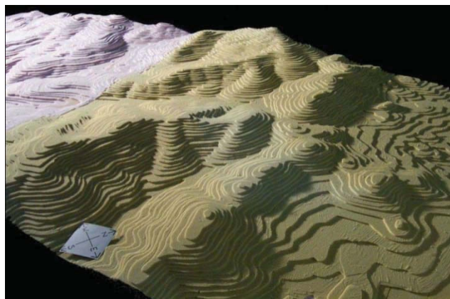
Figure 13-1 Scale model of Altamont Pass used in wind tunnel tests. (Source: Lubitz, W.D. and R.B White, "Prediction of Wind Power Production Using Wind-Tunnel Data, a Component of a Wind Power Forecasting System" (Proceedings of AWEA WindPower 2004))
