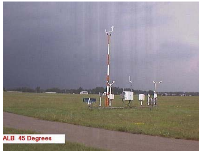
Figure 12-6 The ASOS station at Albany Airport, Albany, New York. (Source: NOAA)
