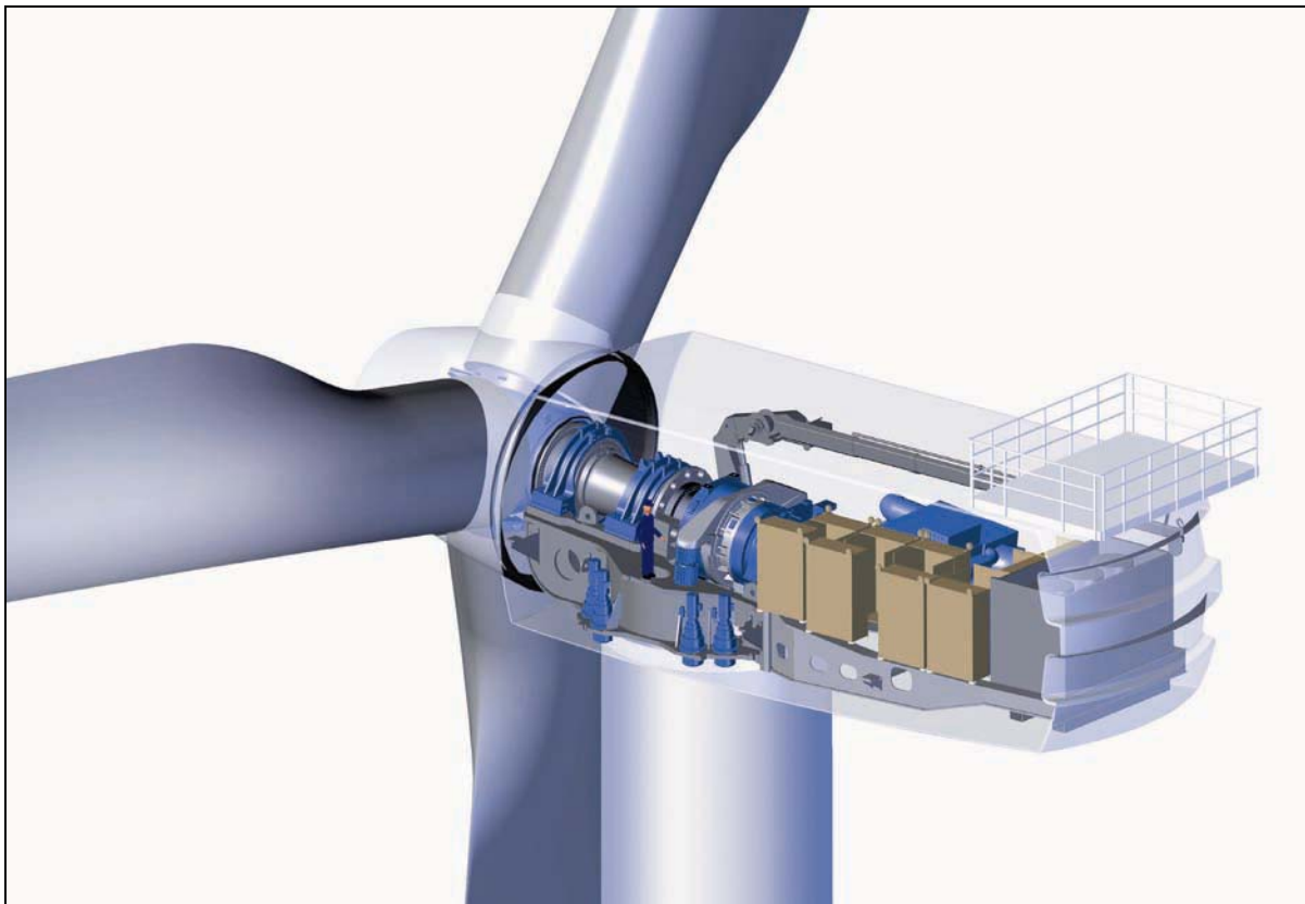
Figure 3.12: Main Components of a Horizontal Axis Wind Turbine 29
