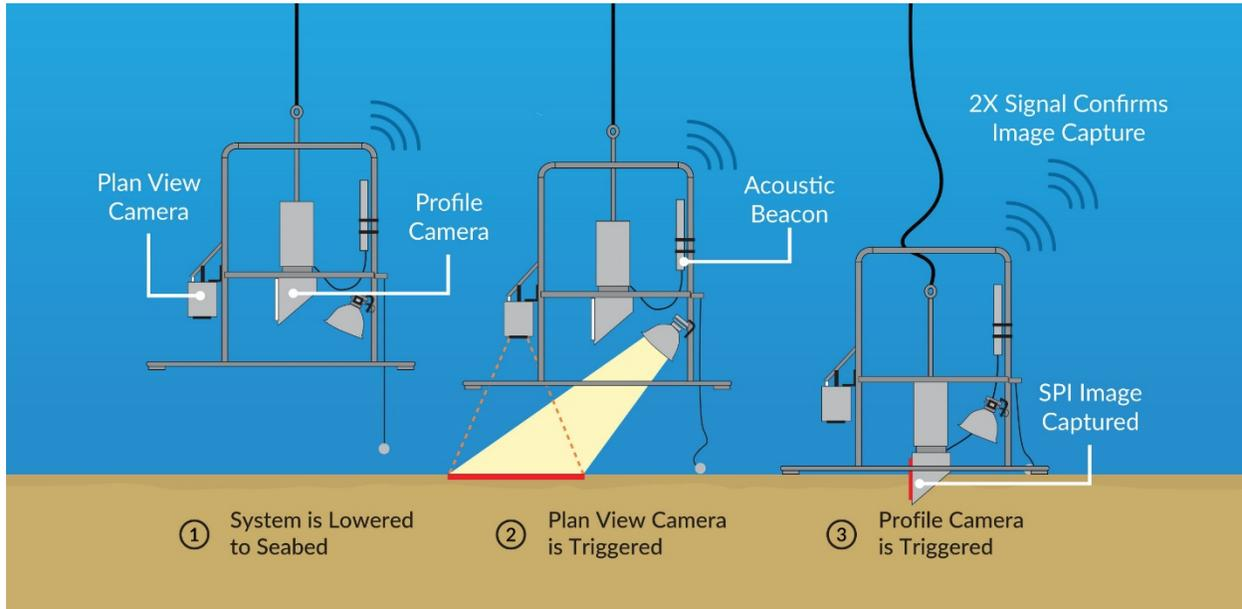
Figure 1. Schematic diagram of SPI/PV deployment
