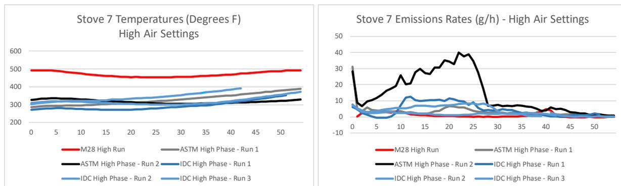
As shown in that figure, the temperature in the M28 high-fire run started out 180°F higher than the highest temperature at the beginning of the high-fire phases of the IDC runs and remained at least 100°F higher than in all IDC runs during the first 30 minutes of the run when most emissions occurred. This may at least partially explain the lower emissions rates for that portion of the M28 run, as shown in the second graph in that figure.
