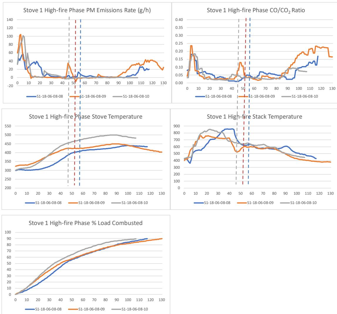
As shown in Figure 110, the high-fire phase PM emission profiles for the stove 1 replicates correlated well with the ratio of carbon monoxide to carbon dioxide (CO/CO<sub>2</sub>) concentrations measured in the exhaust (R squared values are 0.42, 0.53, and 0.50 for runs 1, 2, and 3, respectively). Because CO is a product of incomplete combustion and CO<sub>2</sub> is a product of complete combustion, this ratio is an indication of the instantaneous efficiency of the burn.
