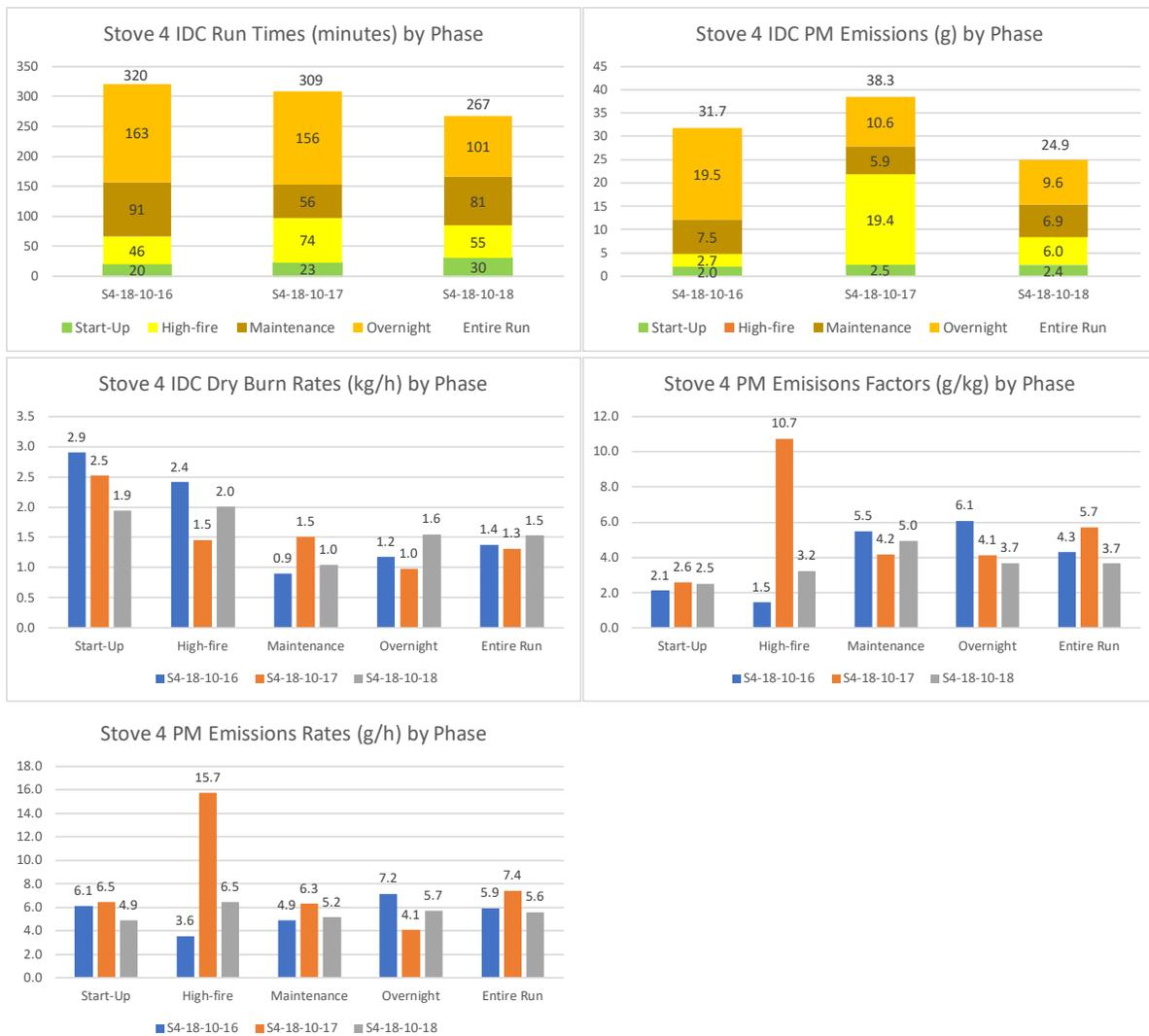
The PM metrics were similar in the three runs with two exceptions: PM emissions were elevated relative to the other runs in run 2 in the high-fire phase and in run 1 in the overnight phase. Figures 117 and 118 show the profiles for the run parameters for those two phases. Again, the time of 50% combustion for each run, when the air setting was moved to low, is shown with dotted lines on the high-fire phase graphs.
