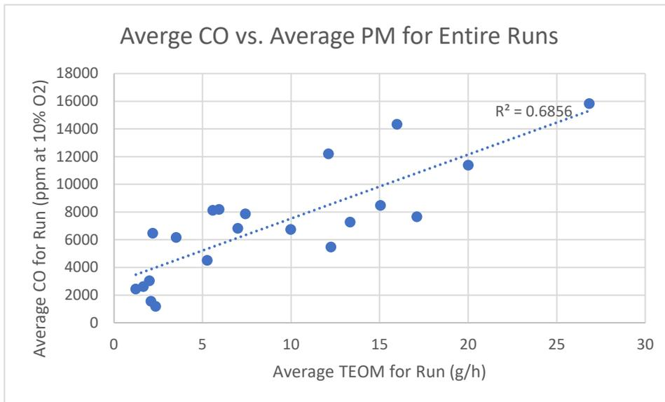
The graphs in Figure 106 show the CO and PM profiles, along with the percent fuel combustion, for each of the runs. Correlations between CO and PM emissions are evident in some of the runs, particularly in stoves 1 and 2. However, while PM emissions tend to be low late in a burn, CO levels increased or remained high late in some phases of runs with stoves 1, 4, 5, and 6.
