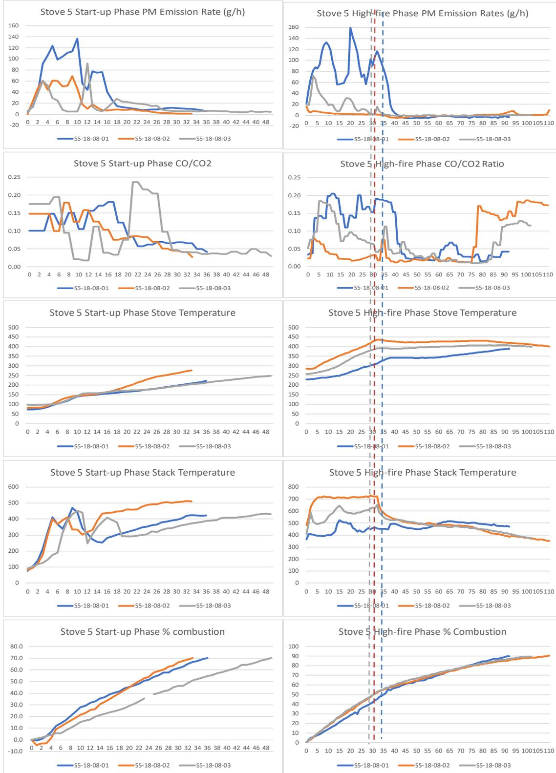
Neither the stack and stove temperatures nor the CO/CO<sub>2</sub> ratio explain why PM emissions in minutes 3–11 of the start-up phase were considerably higher in run 1 (S5-18-08-01) than in the other runs. In that period, stove temperatures in all runs were similar and stack temperatures and the CO/CO<sub>2</sub> ratio in run 1 were within the range of those in the other runs. The run 1 combustion rate was slightly higher than those of the other runs in that period.
