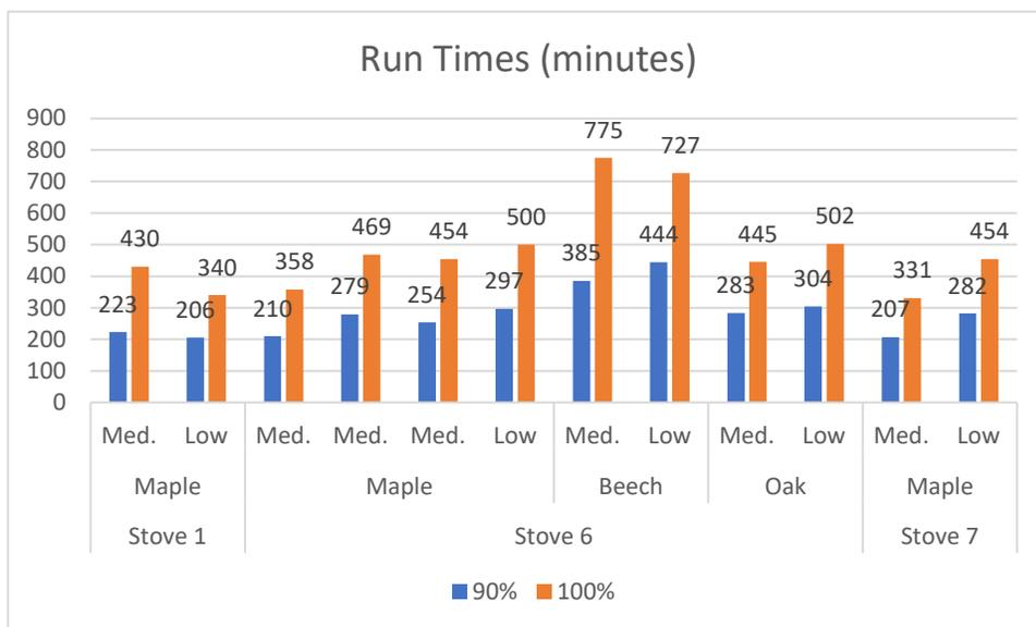
As with the M28 runs, substantial additional time was required to consume the last 10 of the fuel loads in the ASTM medium and low burns, as shown in Figure 68. On average, the 100% fuel consumption periods were 201 minutes longer than the 90% consumption periods. The time period between 90% and 100% fuel consumption constituted an average of 41% (range 36%–50%) of the total run times.
