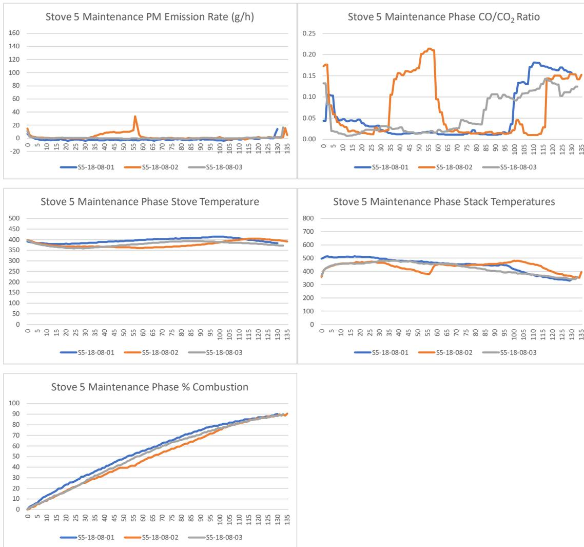
As shown in that figure, the significant PM emissions in the second run, S5-18-08-02, occurred in a 25-minute period beginning at minute 35. In that period, the CO/CO<sub>2</sub> ratio was highly elevated relative to fuel combustion, and stove and stack temperatures were lower than in the other runs. It is not clear what caused the poor combustion conditions, reduced temperatures, and increased higher PM emissions in run 2 relative to the other runs during that 25-minute period.
