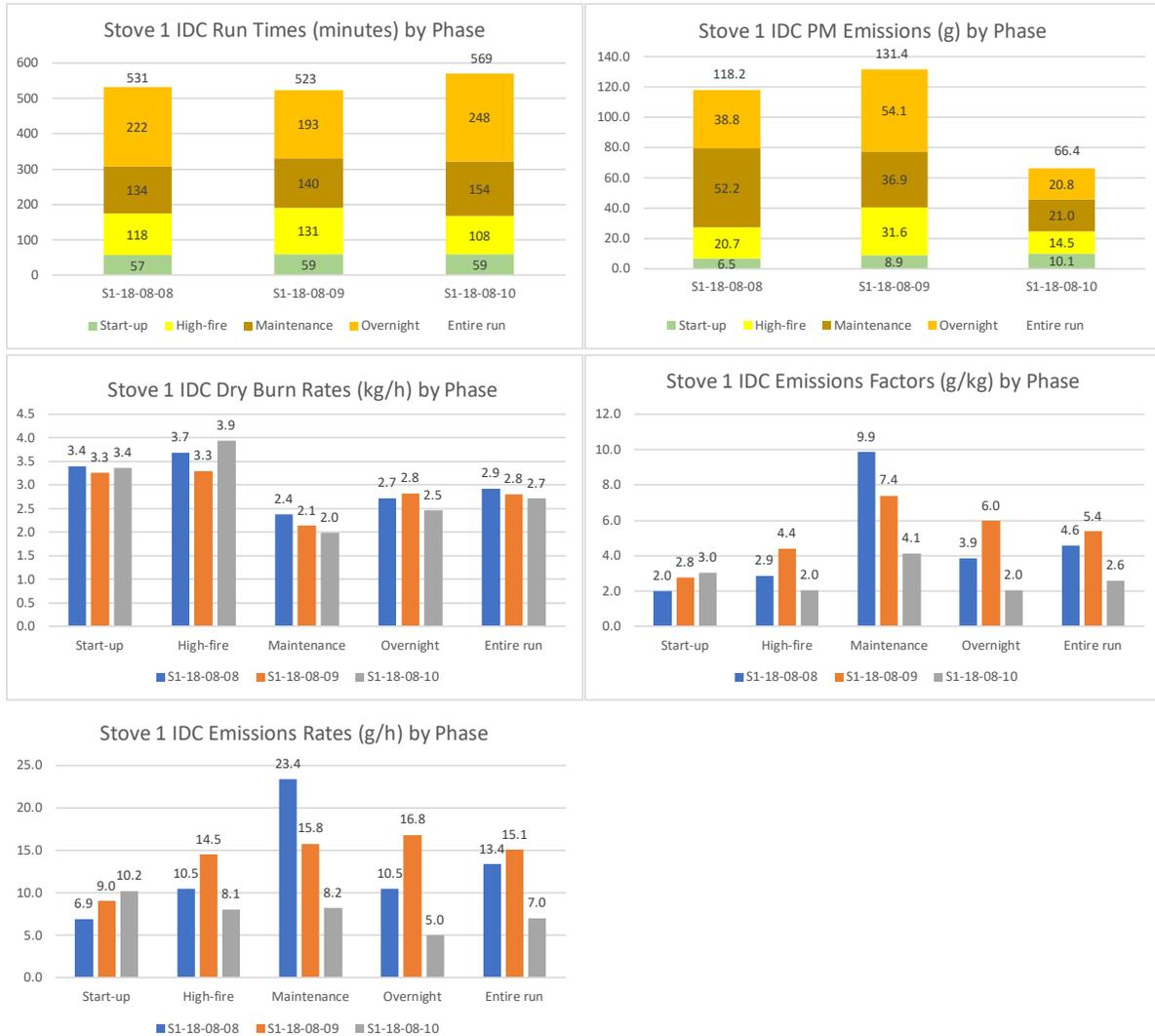
Total PM emissions and the PM EF and ER for all phases except start-up were lowest in S1-18-08-10 (run 3). PM metrics were highest in S1-18-08 (Run 1) in the maintenance phase and highest in S1-18-09 (run 2) in the high-fire and overnight phases. The start-up phase contributed a small percentage of total PM emissions. The analysis below investigates factors that may help explain the PM emission differences in the runs in the high-fire, maintenance, and overnight phases.
