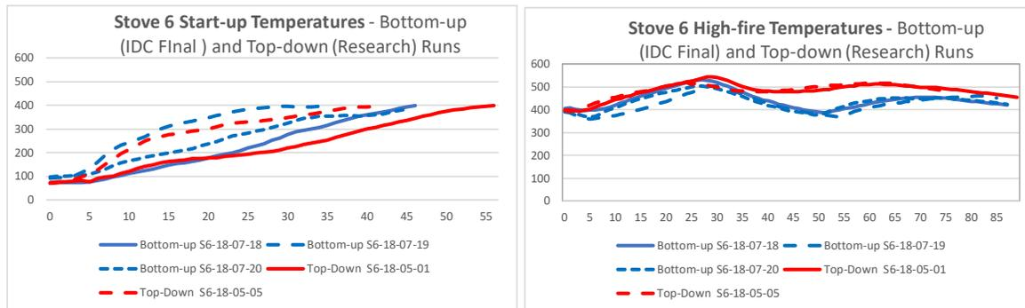
Temperatures in the start-up phase of the bottom-up runs tended to be higher than those in the top-down runs. The temperature difference was most notable in the runs for stove 2 and 5. As shown in Figure 4-11, the higher bottom-up temperatures were, in most cases, associated with higher burn rates and lower run times in the start-up phase.
