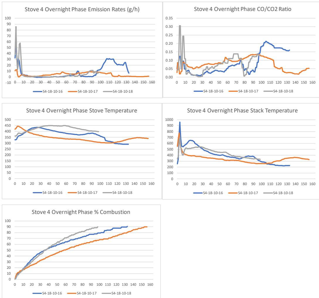
The higher PM emissions measured in run 1 in this phase relative to the other runs primarily occurred at the end of the run, beginning at minute 92 and peaking at minute 110. During that period, run1 stove and stack temperatures and the fuel combustion rate decreased and the CO/CO<sub>2</sub> ratio increased, while the reverse was true for run 2. Run 3 ended shortly into that period.
