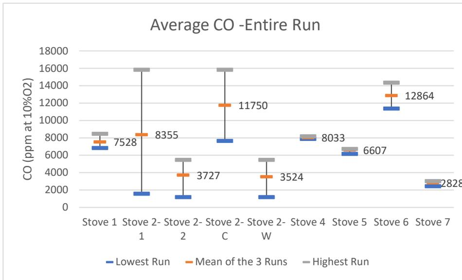
Stove 2 results are grouped in two ways, the initial set of three replicates and according to the initial door position, cracked (denoted above as C) or wide open (W).
