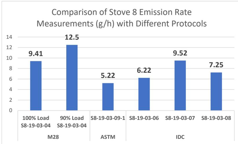
As shown in that figure, for stove 8, the ER measured with M28 was within the range of those measured using the IDC protocol and the ASTM 3053-17 result was below that range.
