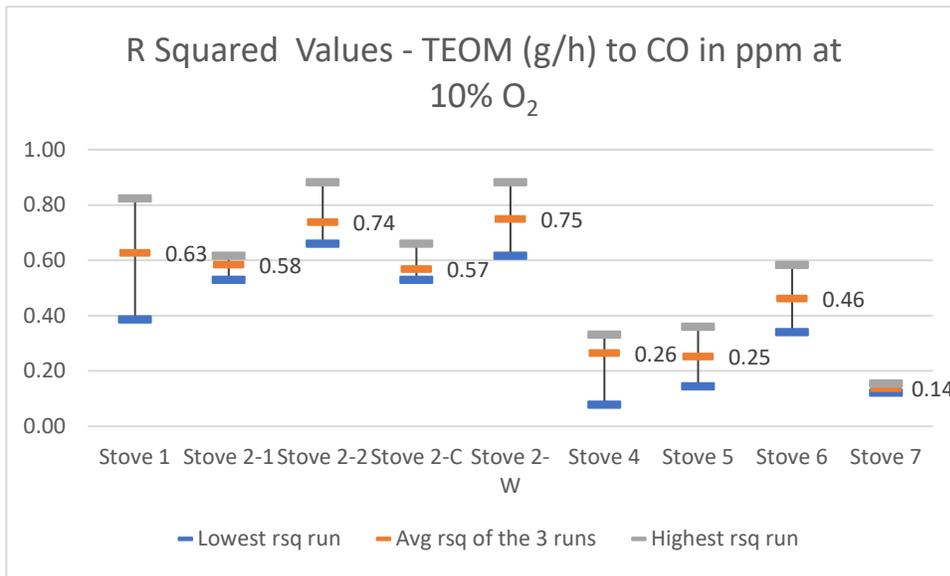
The average CO correlated well ( $r^2 = 0.69$ ) with average PM<sub>2.5</sub> (TEOM measurement for entire runs, as shown in Figure 105). Stoves with low PM<sub>2.5</sub> emissions (e.g., stove 7) also had lower CO emissions.
