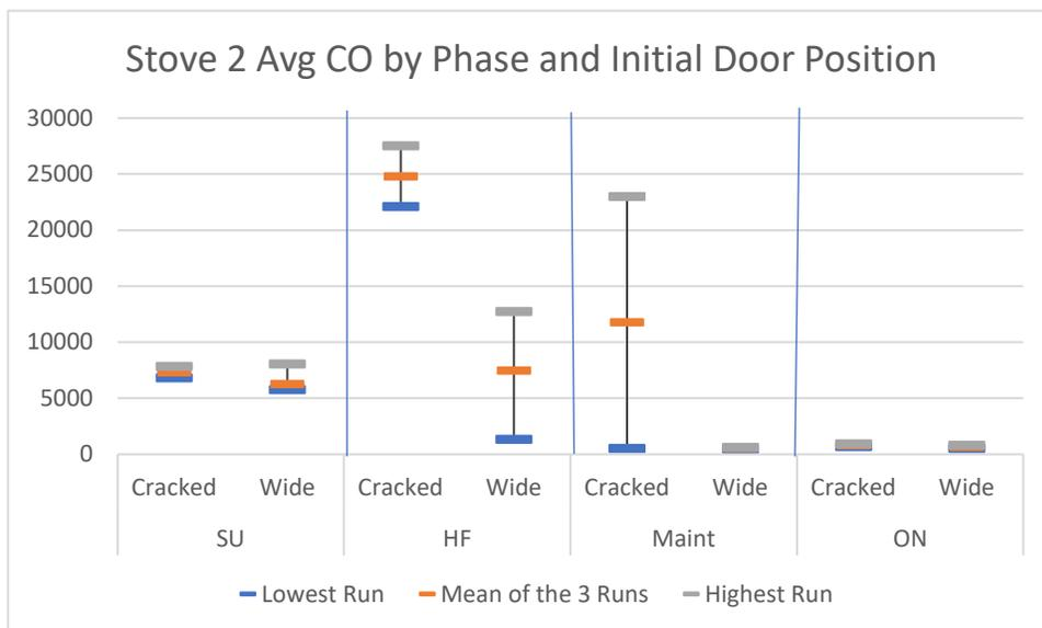
Start-up (SU) CO emissions were similar in all stove 2 runs. High-fire (HF) phase CO was considerably higher in all of the runs with the door initially cracked open than in the wide-open door runs. The higher CO levels carried over to the maintenance phase in one of the cracked-open runs. CO emissions in the maintenance phases of the other stove 2 runs and in the overnight phases of all of the stove 2 runs were low.
