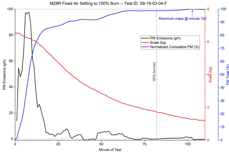
\* Real-time PM Measurements obtained with Teom. On average Teom measurements are 10% less than filter measurements.
