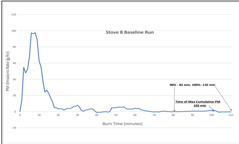
Note that the scales in the Figure 74 graphs are very different. Stove 1, the only large stove in this group, and stove 8, the fixed-air setting stove, had a considerably higher peak PM emission rate than the other stoves, while the instantaneous emission rates for stove 7, the stove with hybrid controls, were the lowest for all burn levels.
