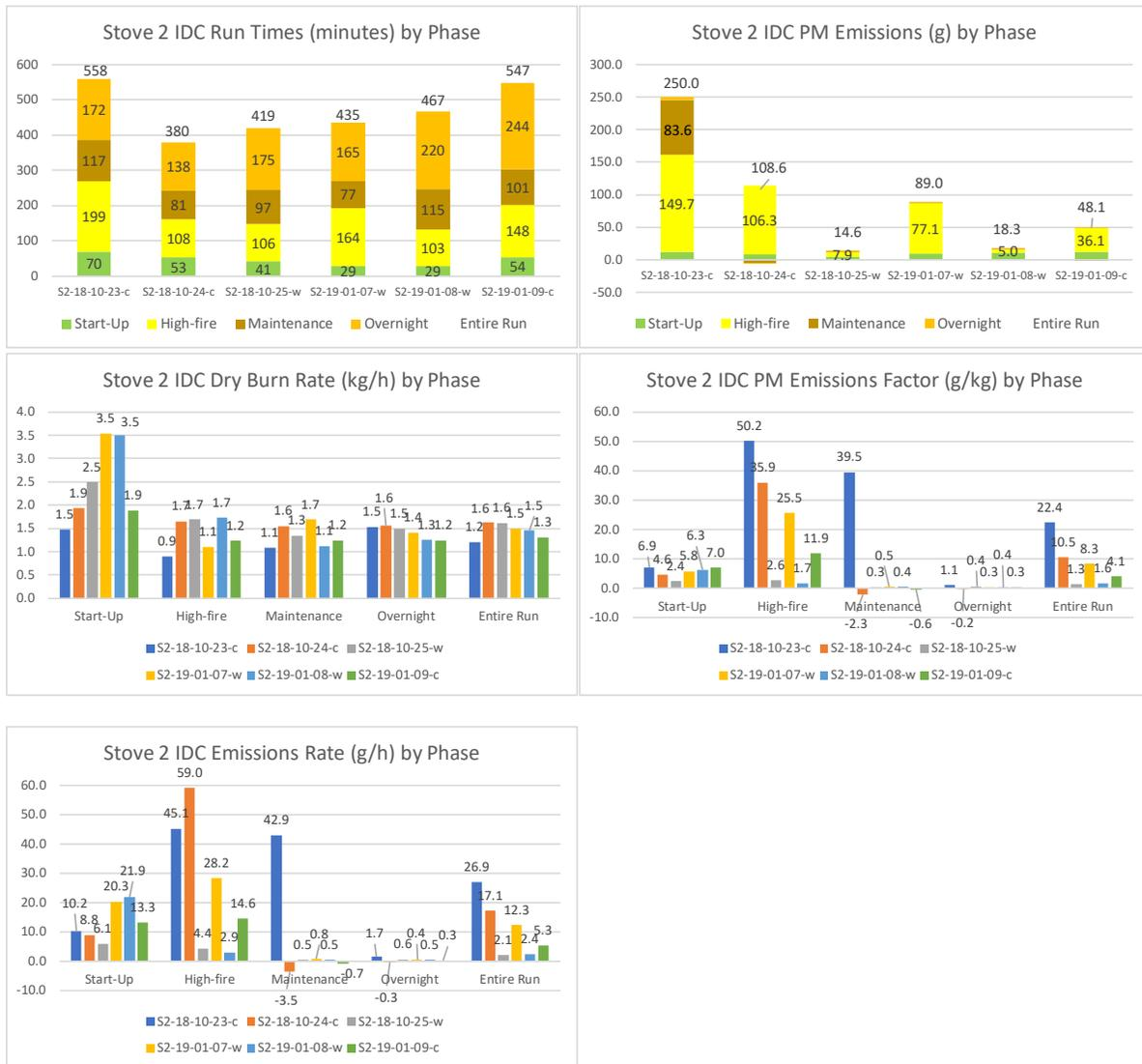
The wide-open door position in the first five minutes of the start-up runs was associated with a higher burn rate in the start-up phase and may have increased the ER in that phase. However, the increased open door start-up phase ER was primarily due to the shorter test times, rather than increased PM emissions, and did not affect the overall ER for entire run. Therefore, it does not appear that the initial door position is an important factor in emission test results.
