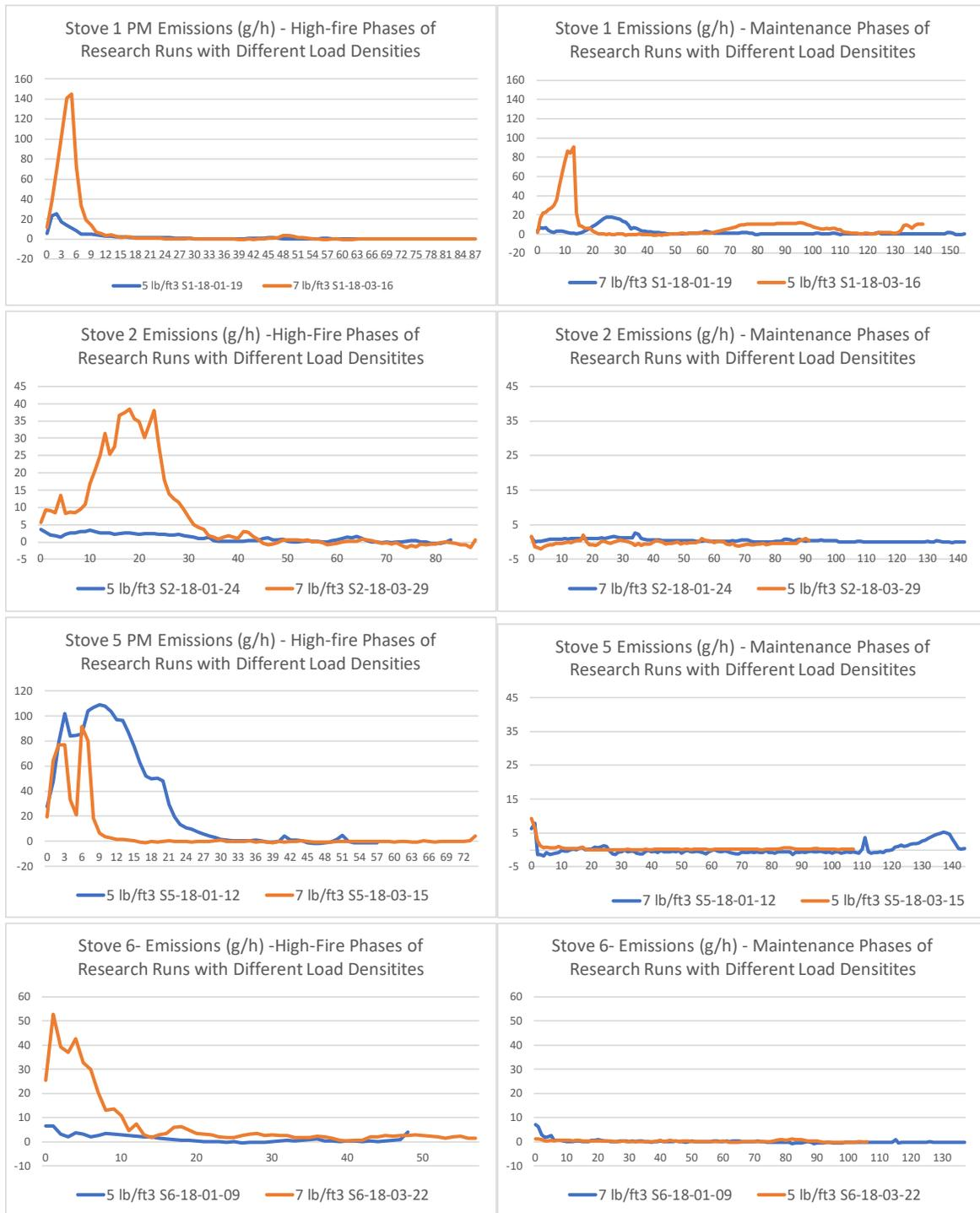
Apart from the stove 5 results, the high-fire phase results support the conclusion that higher density loads tend to produce higher PM emissions in that phase. Because the maintenance phase tended to produce minimal emissions, a test with the higher density load in the high-fire phase rather than the maintenance phase is more likely to be associated with higher emissions for those two phases combined.
