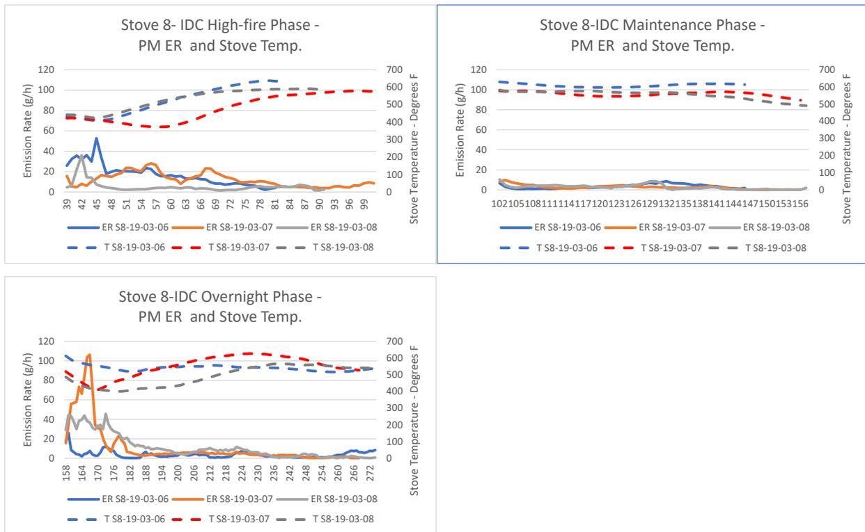
Temperatures remained well above 500°F throughout most of the maintenance phase in all runs, which may explain the consistently low emissions in that phase. In the overnight phase, the initial temperature in run S8-19-03-06 was 94°F to 126°F higher than in the other runs, which may explain the relatively low-PM emissions in that run. The temperature profiles do not explain the inter-run differences in the emission patterns in the high-fire phase.
