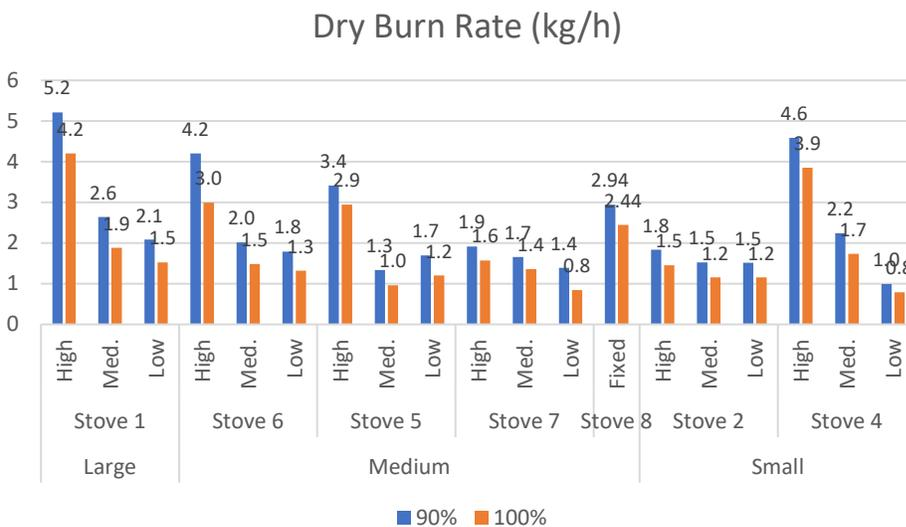
Fuel combustion rates tended to be higher in the larger stoves. However, the high-burn run, fuel combustion rate for stove 4, which has the smallest firebox, was second only to that of stove 1, the largest stove.
