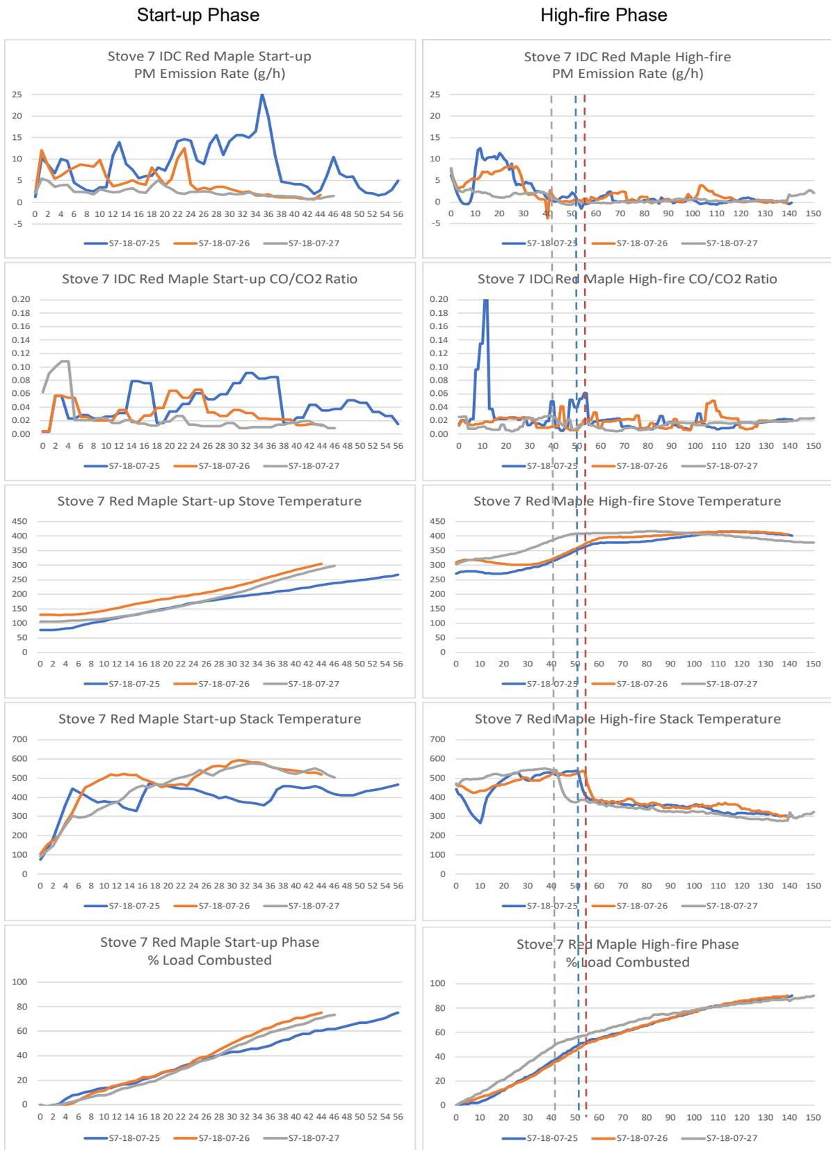
As with previous stoves, the above factors do not give much insight into PM emissions early in the start-up phase. However, the higher PM emissions in run 1 in the second half of that phase correlated with a higher CO/CO<sub>2</sub> ratio and lower stove and stack temperatures and fuel consumption rate relative to the other runs in that period.
