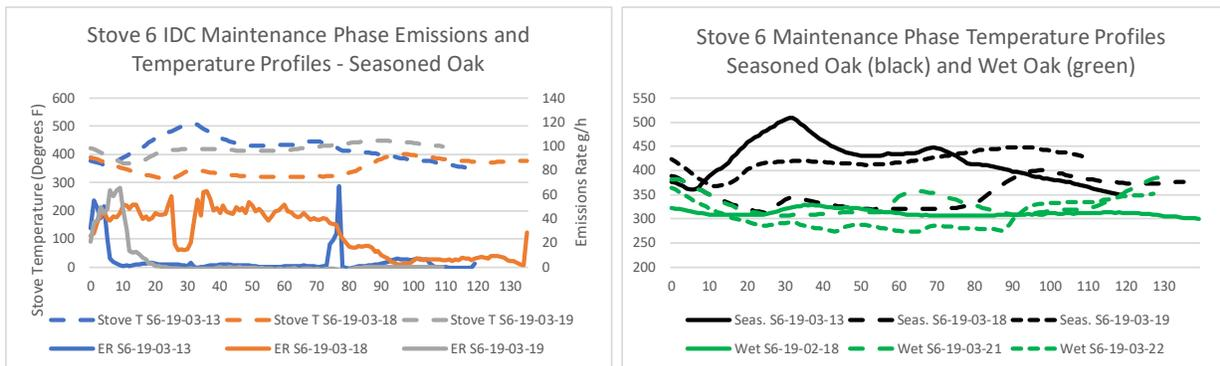
The final phase of the IDC protocol represents a long burn, such as an overnight burn or a burn during the day when the fire will be unattended for a significant amount of time. During this phase, the coal bed is raked, and the user loads as much wood as possible, using large and small pieces. The metrics measured in the overnight phase of the stove 6 IDC runs are shown in Table 106.
