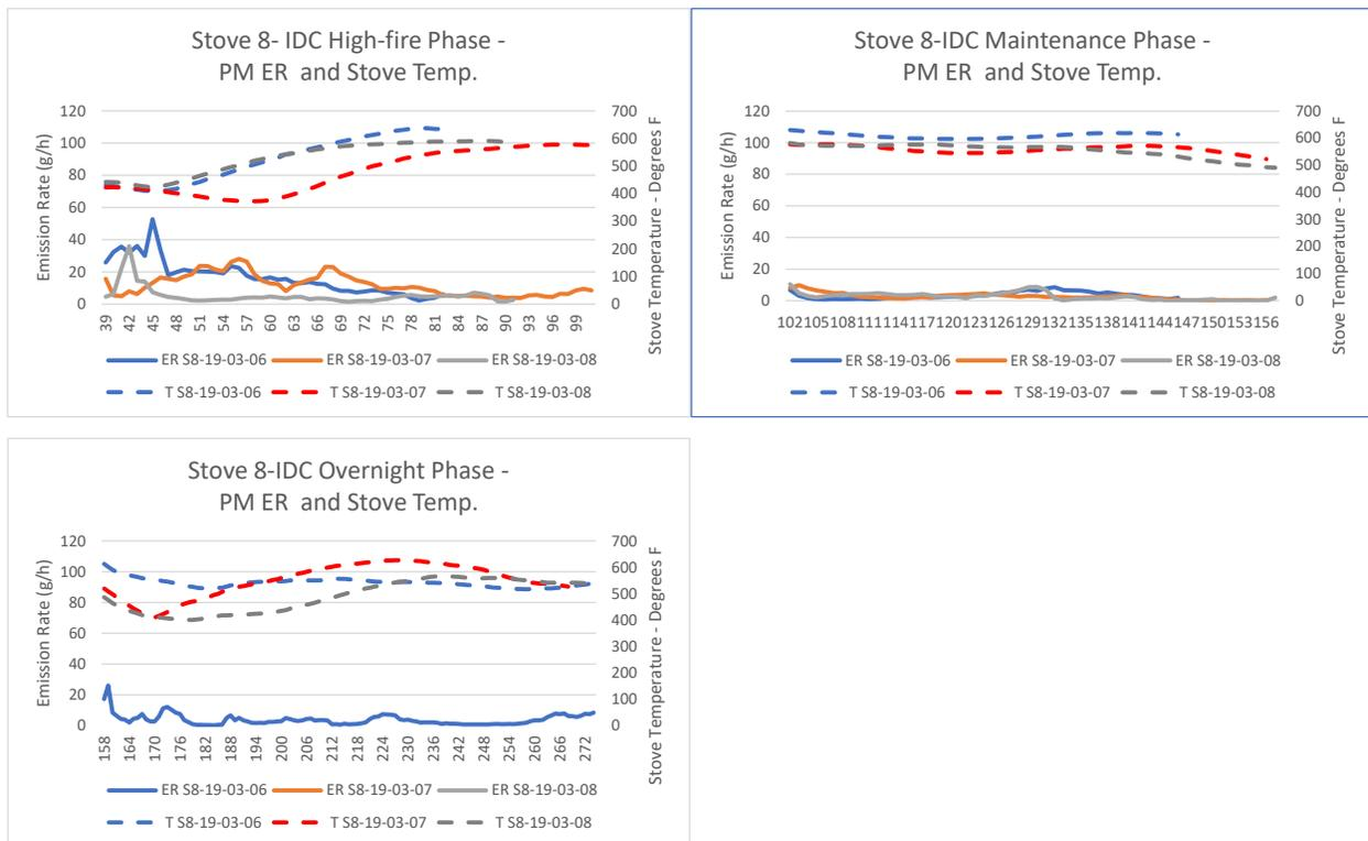
The temperature profiles do not explain the inter-run differences in the emission patterns in the high-fire phase. Temperatures remained well above 500°F throughout most of the maintenance phase in all runs, which may explain the low emissions in that phase. In the overnight phase, the initial temperature in run S8-19-03-06 was 94°F to 126°F higher than in the other runs, which may explain the relatively low PM emissions in that run.
