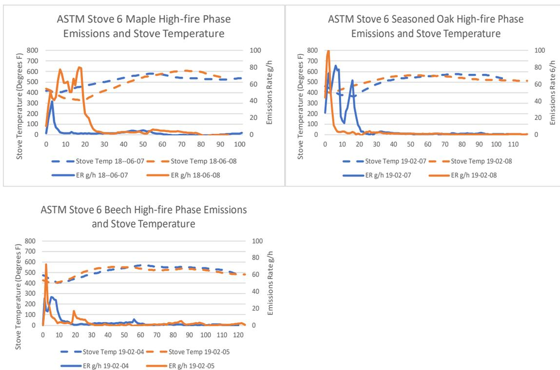
The ASTM 3053-17 high-fire phase ends when 90% of the fuel load is consumed. At that point, the stove is moved to the air setting for the next phase for an hour. At the end of the hour, a full charge of 12 lb/ft<sup>3</sup> is reloaded and a low- or medium-fire burn is conducted. The metrics for the three low fire phase burns (one with each wood species) are shown in Table 100.
