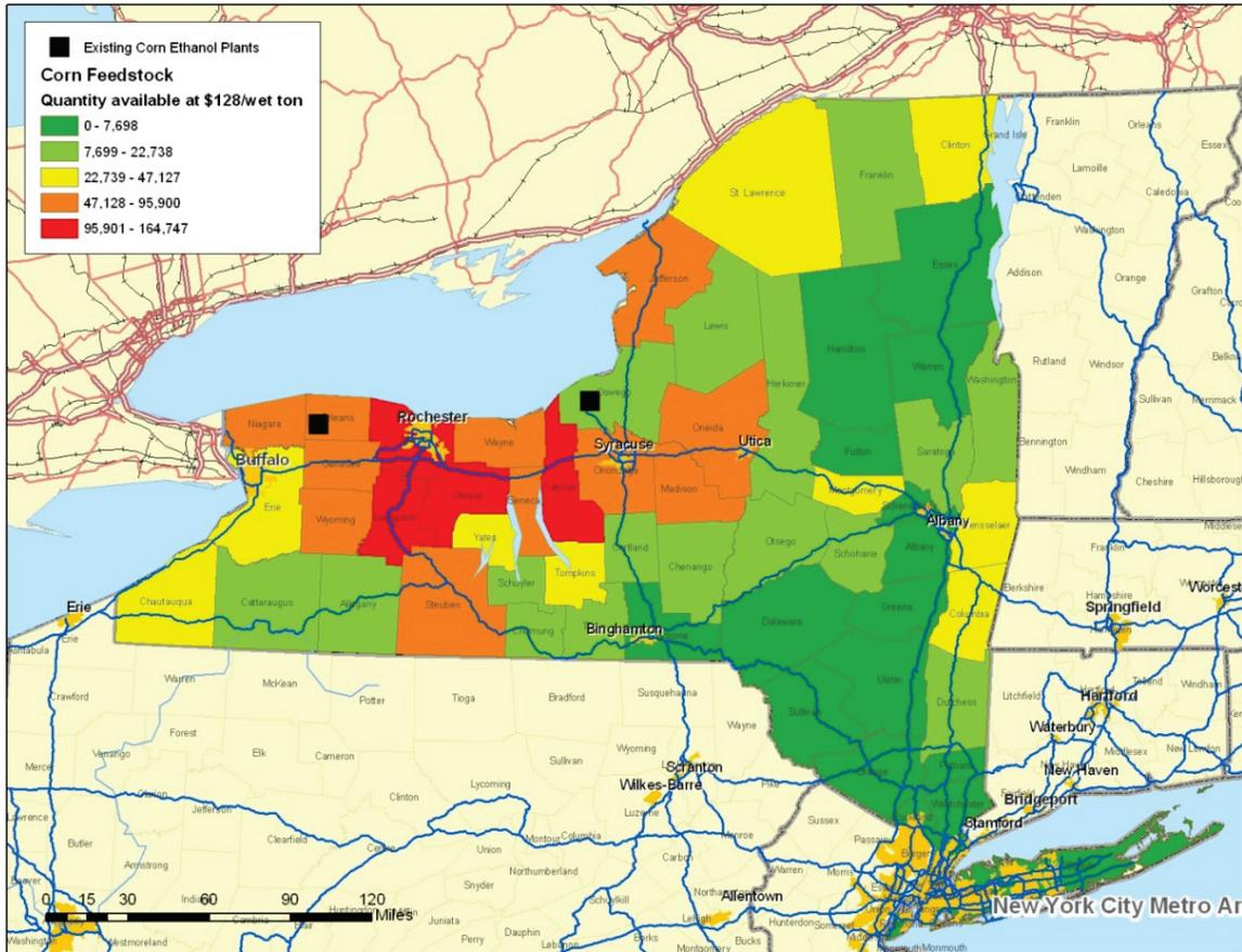
The operating grain ethanol biorefinery draws 80% of its total supply of corn from in-state. It was assumed that all feedstocks would come from within New York. In addition, counties were allocated to each biorefinery on the basis of shortest transportation routes, and transportation hauling mileages and costs were calculated accordingly.
