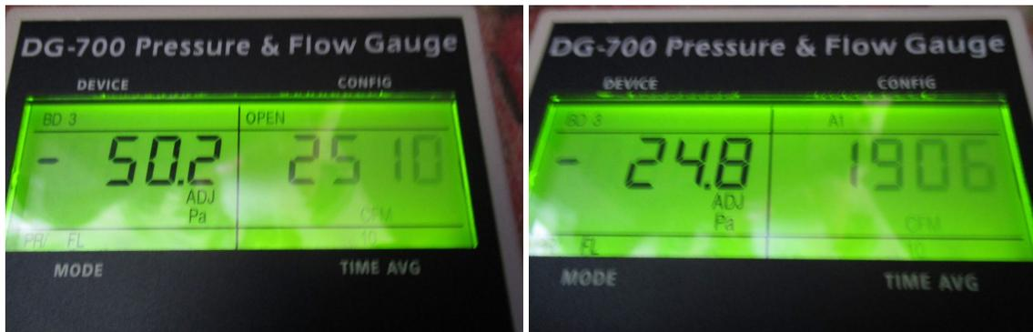
Blower door testing creates exaggerated pressure differences between the inside and outside of a structure in order to measure air leakage. Indiscriminate use of blower door equipment in homes with combustion appliances and/or that contain hazardous materials (such as asbestos or mold) may create unsafe conditions inside a home. Accordingly, Cadmus did not perform a blower door test where the technician encountered one or more of these conditions onsite:
