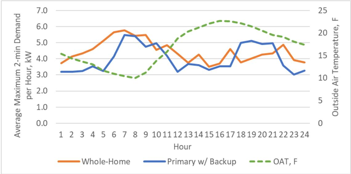
**Figure 5. Cold Snap Average Site Heating Performance**
