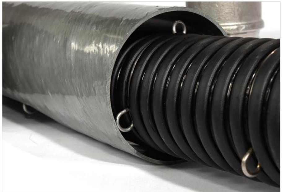
The outer pipe is patented, low-thermal resistance composite material. The center flow channel is heavy duty, nylon-reinforced EDPM corrugated rubber which provides turbulent flow and thermal separation between fluid steams.
