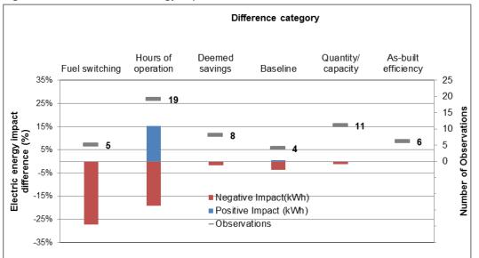
Figure 4-3. ADEEP Electric Energy Impact – Sources of Realization Rate Differences
