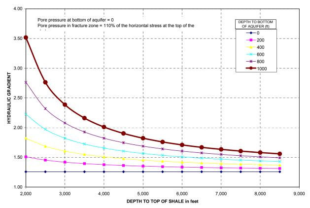
Figure 1: Average hydraulic gradient during fracturing
