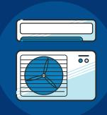
Air source heat pumps extract heat from outside air that is then used for heating indoor spaces during the colder months. They can also extract heat from indoors and expel it outside to cool indoor spaces during the warmer months. Air source heat pumps can be used to heat or cool single rooms (partial load) and whole homes (full load).
