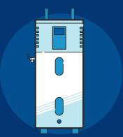
Heat pump water heaters extract heat from the air surrounding the unit to heat water. They can replace electric or fossil fuel-powered water heaters that require much more energy to run efficiently leading to big savings.
