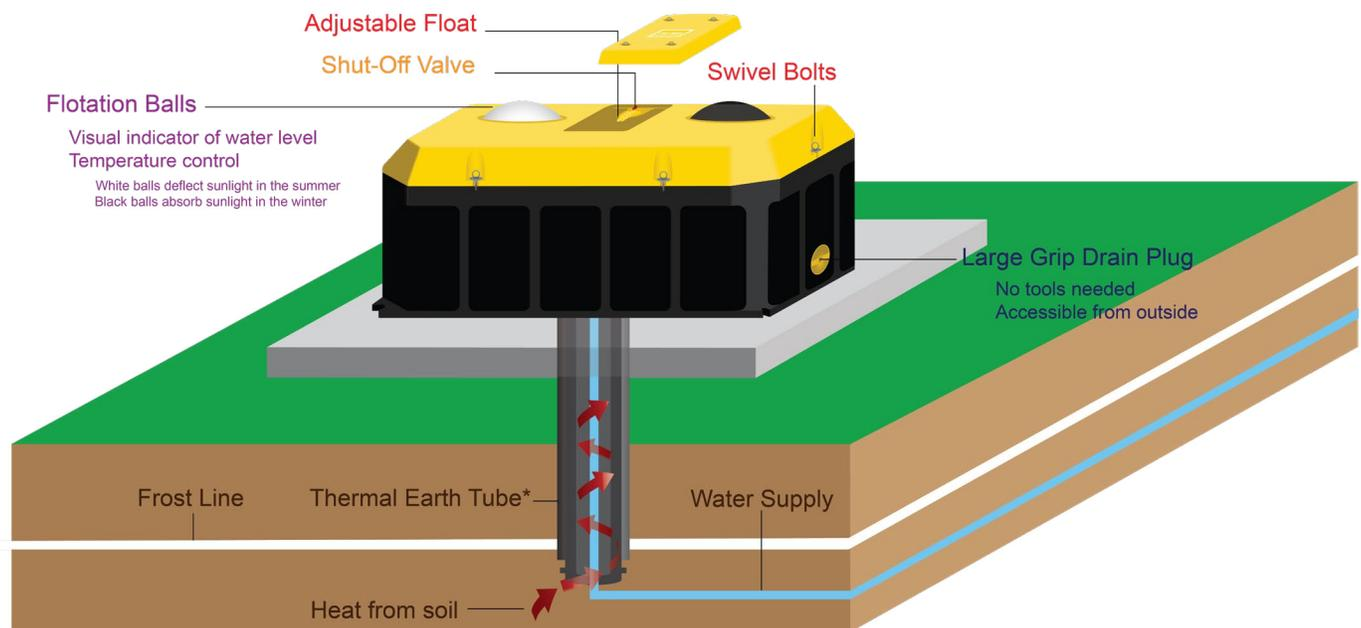
\*To prevent your vertical water supply line from freezing, an insulated thermal earth tube is installed under the ground during set-up.
