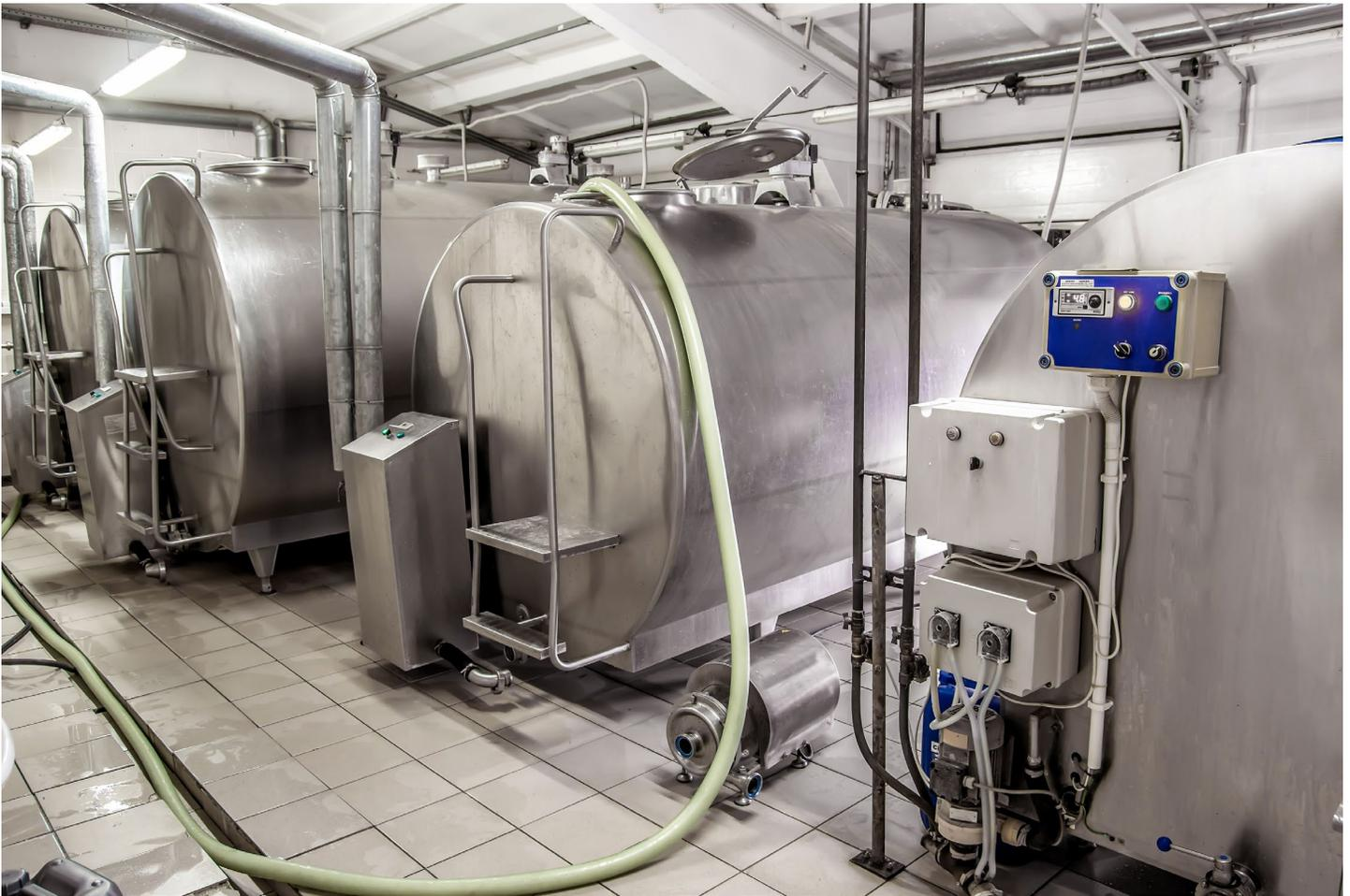
Milk Bulk Tank with a Built-In Refrigeration System.
