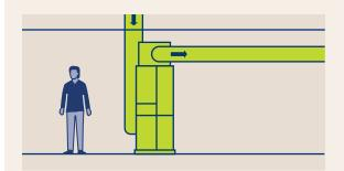
Conventional air handlers move air through larger ducts. They are often located in basements, attics, or utility closets. They can be installed to blow air upwards, downwards, or sideways to fit within your home.
