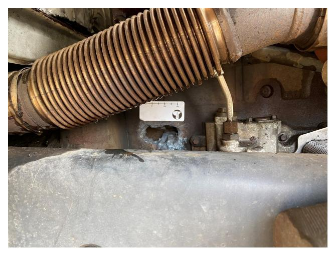
6. Engine destruction - a photograph of the 3-inch hole in the engine and NYTVIP supplied sticker from a few feet back that also includes some truck/bus color.
