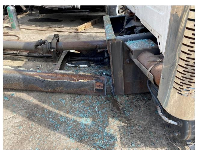
7. Cut chassis - a close-up of the cut chassis that includes some color of the truck/bus.
