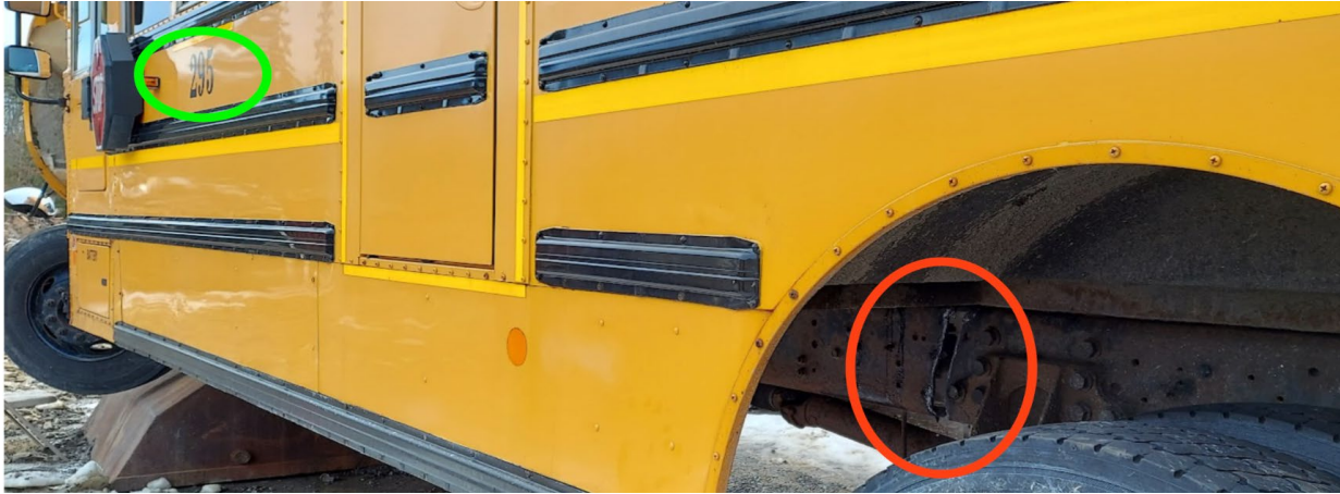
Figure 14. The “after” photos of the left side of a school bus whose left frame rail has been cut (orange highlight) and documented with the identifying number of the vehicle (green highlight).
