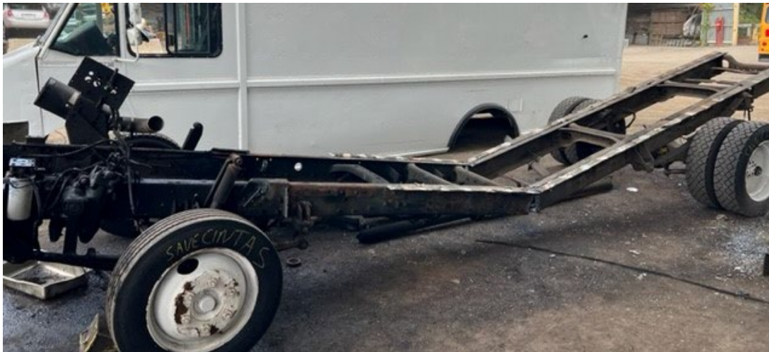
Figure 13. An “after” photo of a cut chassis from a van, with its body alongside.
