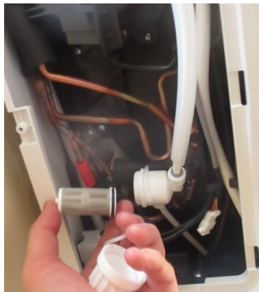
Figure 17. Improved Inline Filter Arrangement: Midea America Production Model
