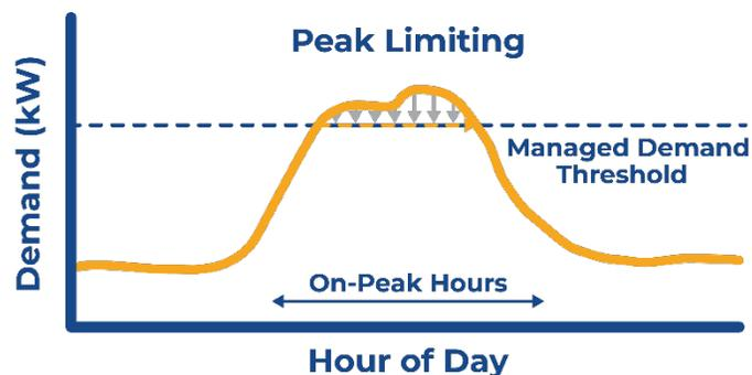
Load shedding entails reducing or turning off loads during the on-peak hours to keep the aggregated demand below the preset level. The candidates for shedding should only be loads that can be reduced or turned off without affecting occupant safety, loads that will not lead to an unrecoverable impact on
