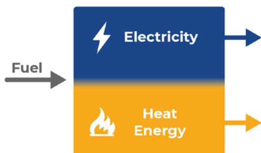
Usually, this requires the energy produced by the waste heat of the CHP plant to be consumed completely in support of building functions. A CHP plant’s overall efficiency when its waste heat offsets another fuel usage can be in the range of 80% to 85%.<sup>1</sup>
