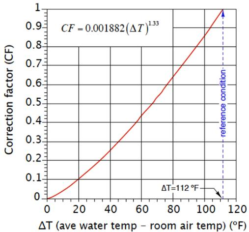
As an approximation, a panel radiator operating with an average water temperature of 110 °F in a room maintained at 68 °F, provides approximately 27 percent of the heat output it yields at an average water temperature of 180 °F.
