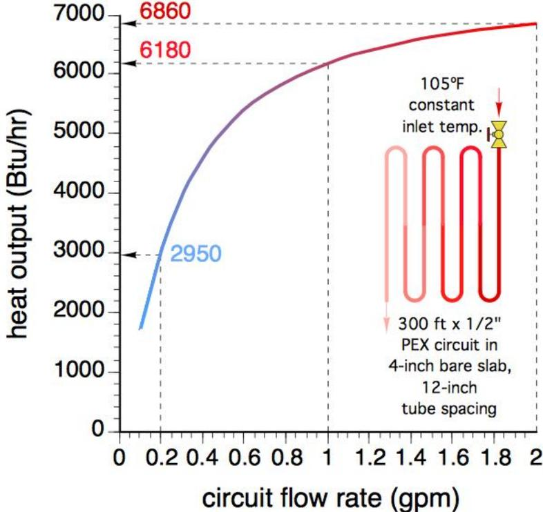
Note diminishing gain in heat output at higher flow rates
