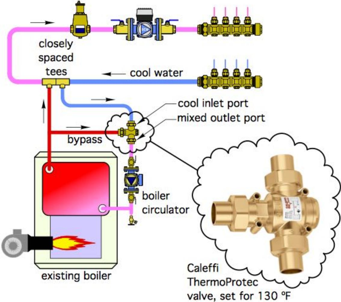
**Keep low temperature heat source “upstream” of existing higher temperature heat source.**
