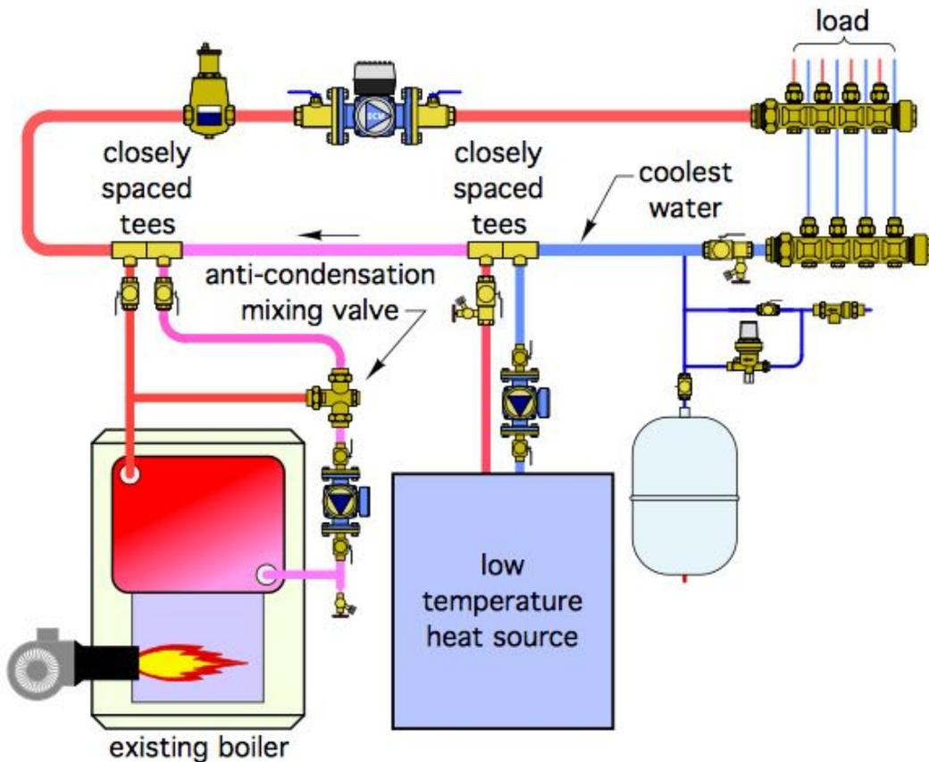
**Allow the coolest water returning from the load to be available to the low temperature heat source.**
