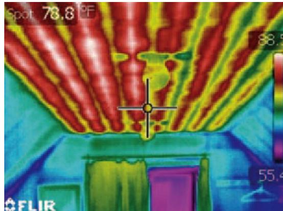
Thermal image of radiant ceiling in operation
