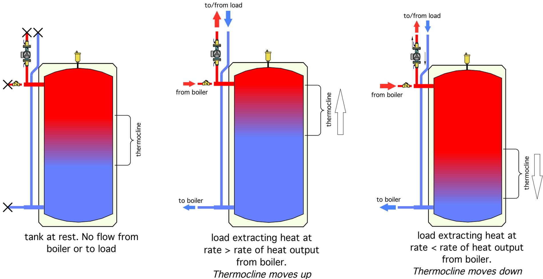
The pellet fired boiler should be turned on **before** the hot water is depleted from top of tank.
