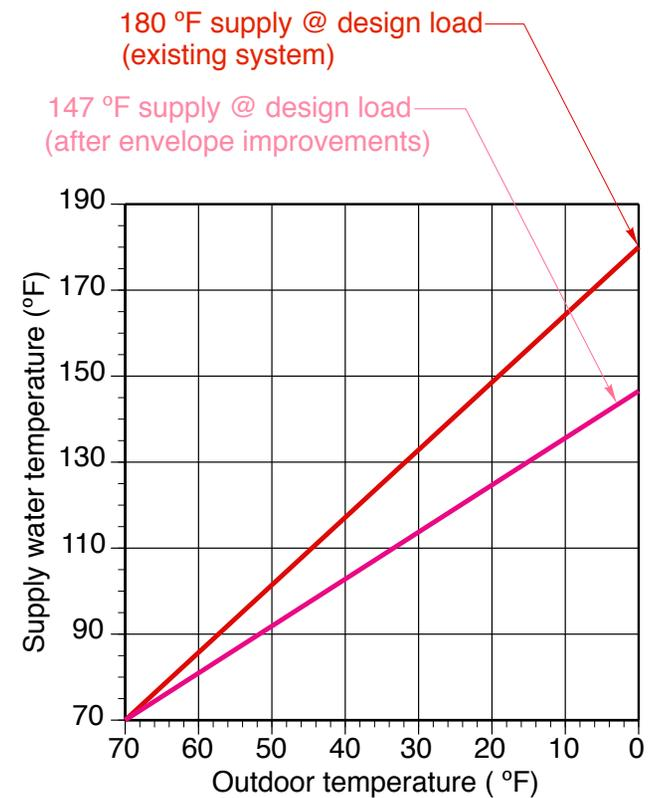
Assume a fin-tube baseboard system (after building envelope improvements) requires 147 °F supply water temperature at design load.
