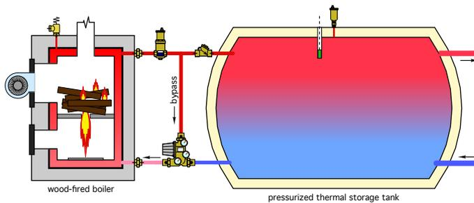
To achieve **high thermal efficiency** and **low emissions**, pellet boilers should operate with long on-cycles, followed by long off-cycles.
