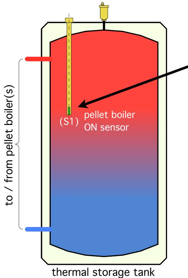
Sensor in vertical well detects “arrival” of rising cooler water. Turns on pellet fired boiler.
