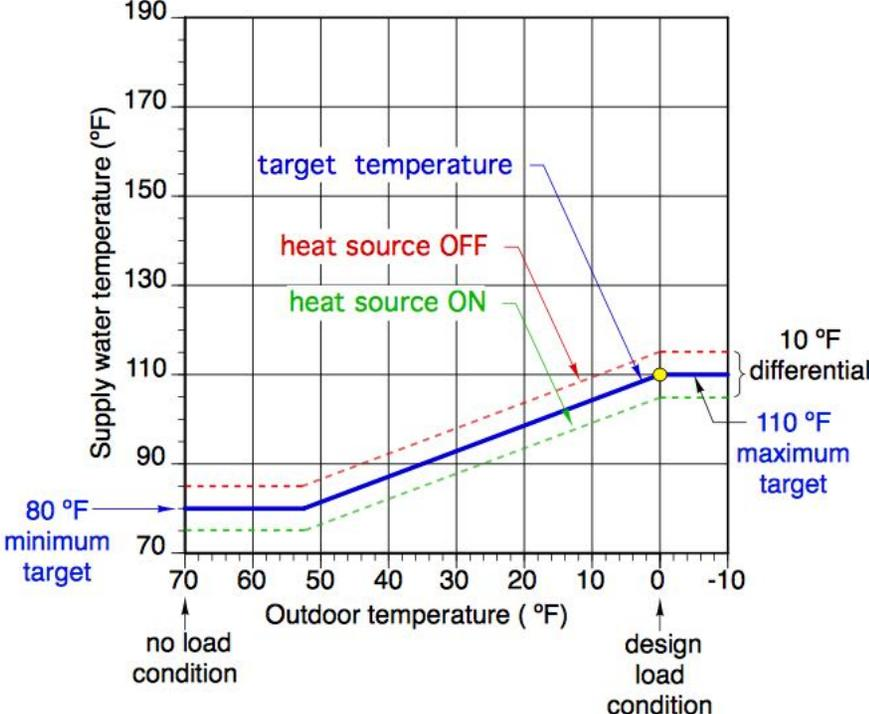
**Typical for heated floor slab**
