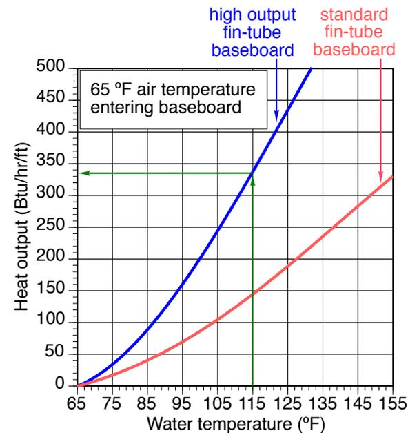
Although this is a reduction compared to the 154 feet of added baseboard required in the previous example, it is still a substantial length. The building must be carefully evaluated to see if this additional length of baseboard can be accommodated.
