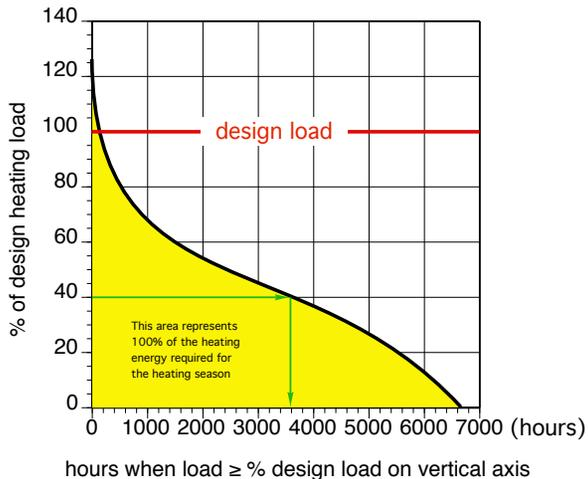
**In this case only 6.5% of heating energy use needs water over 120 °F**
