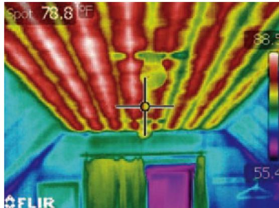
Thermal image of radiant ceiling in operation
