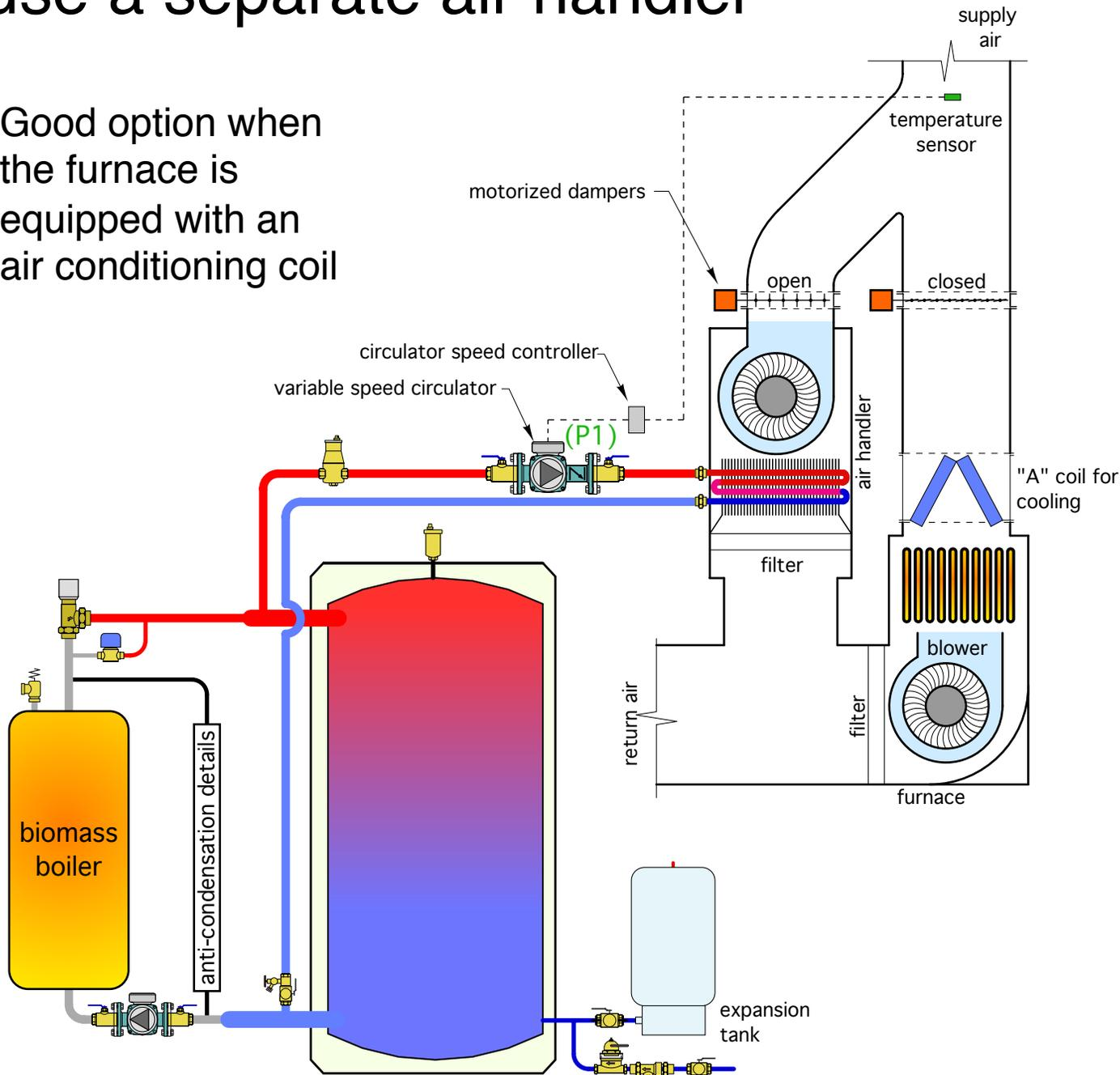
Example of an air handler with hydronic coil
