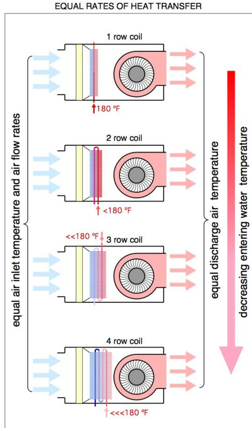
However, “deeper” coils (w/ more tube rows) create higher static pressure losses in the forced air system.
