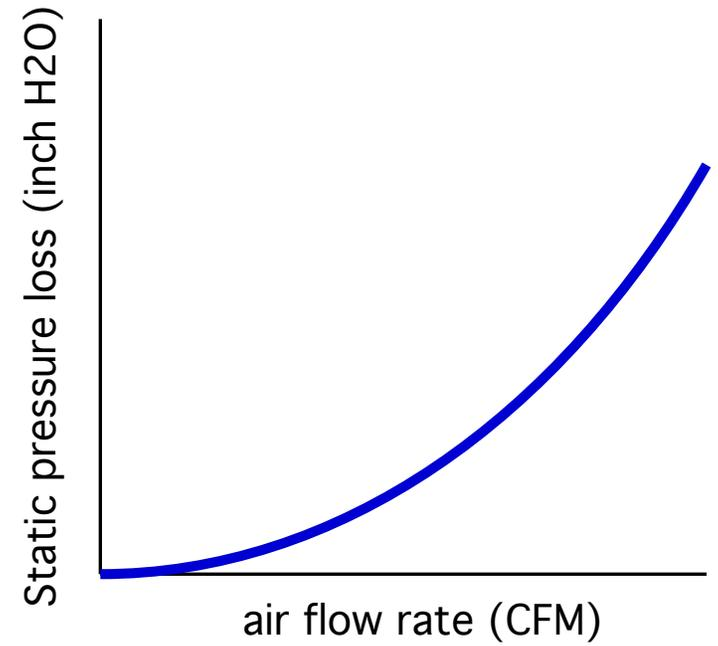
Get  $\Delta P$  vs. air flow rate data for specific coil from manf.
