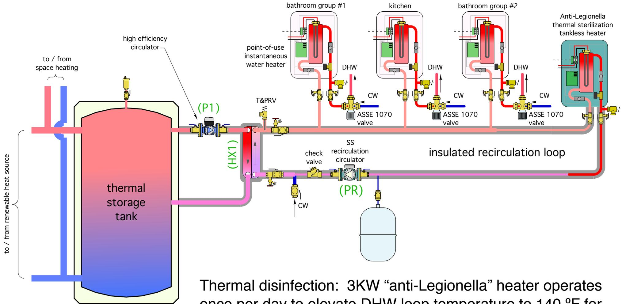
Thermal disinfection: 3KW “anti-Legionella” heater operates once per day to elevate DHW loop temperature to 140 °F for 30 minutes. This cycle is typically at night.
