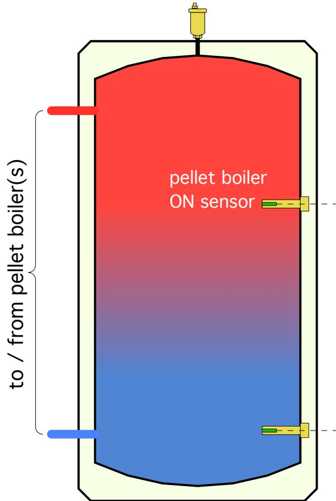
Pellet boiler fired when UPPER tank sensor drops to the target temperature of the outdoor reset controller
