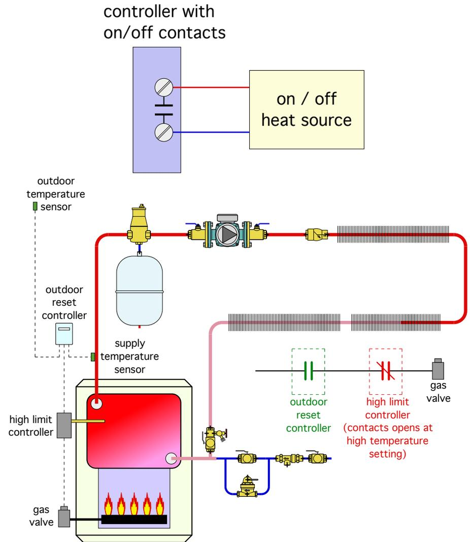
**Design tip: Setting the minimum supply water temperature to 140 °F on conventional gas-fired boilers will generally provide anti-condensation protection.**
