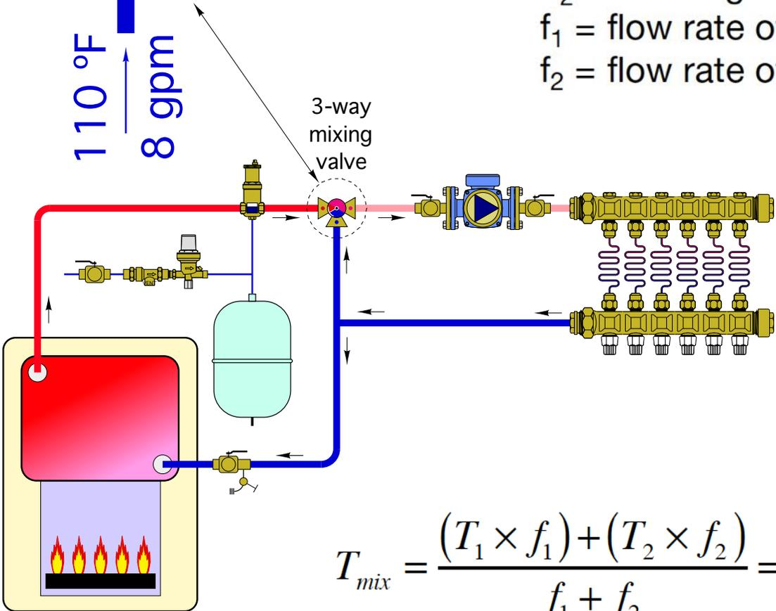
$$T_{mix} = \frac{(T_1 \times f_1) + (T_2 \times f_2)}{f_1 + f_2} = \frac{(170 \times 5) + (110 \times 8)}{5 + 8} = 133^\circ F$$
