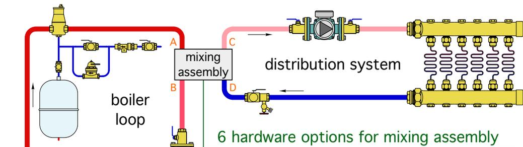
The 3-way motorized mixing valve, or variable speed injection pump methods of mixing are most appropriate for biomass boiler systems the most appropriate.
