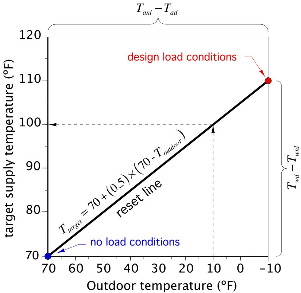
$$RR = \frac{(T_{wd} - T_{wnl})}{(T_{anl} - T_{ad})} = \frac{(110 - 70)}{(70 - [-10])} = \frac{40}{80} = 0.5$$
