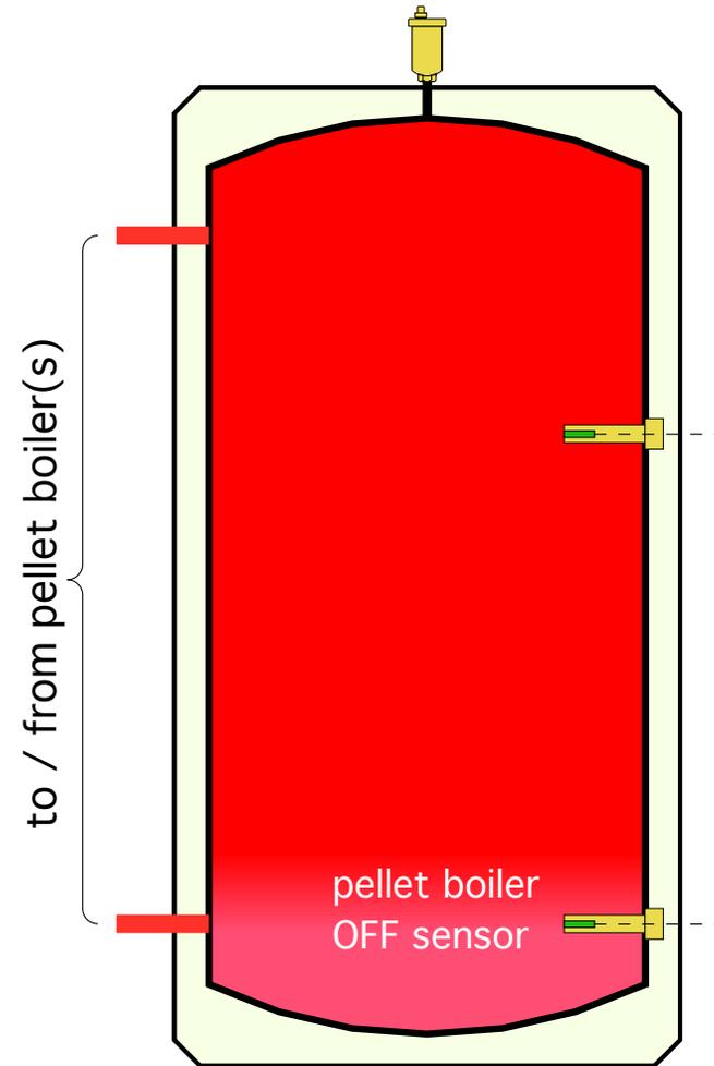
Pellet boiler turned off when LOWER tank sensor climbs to some higher setpoint temperature.
