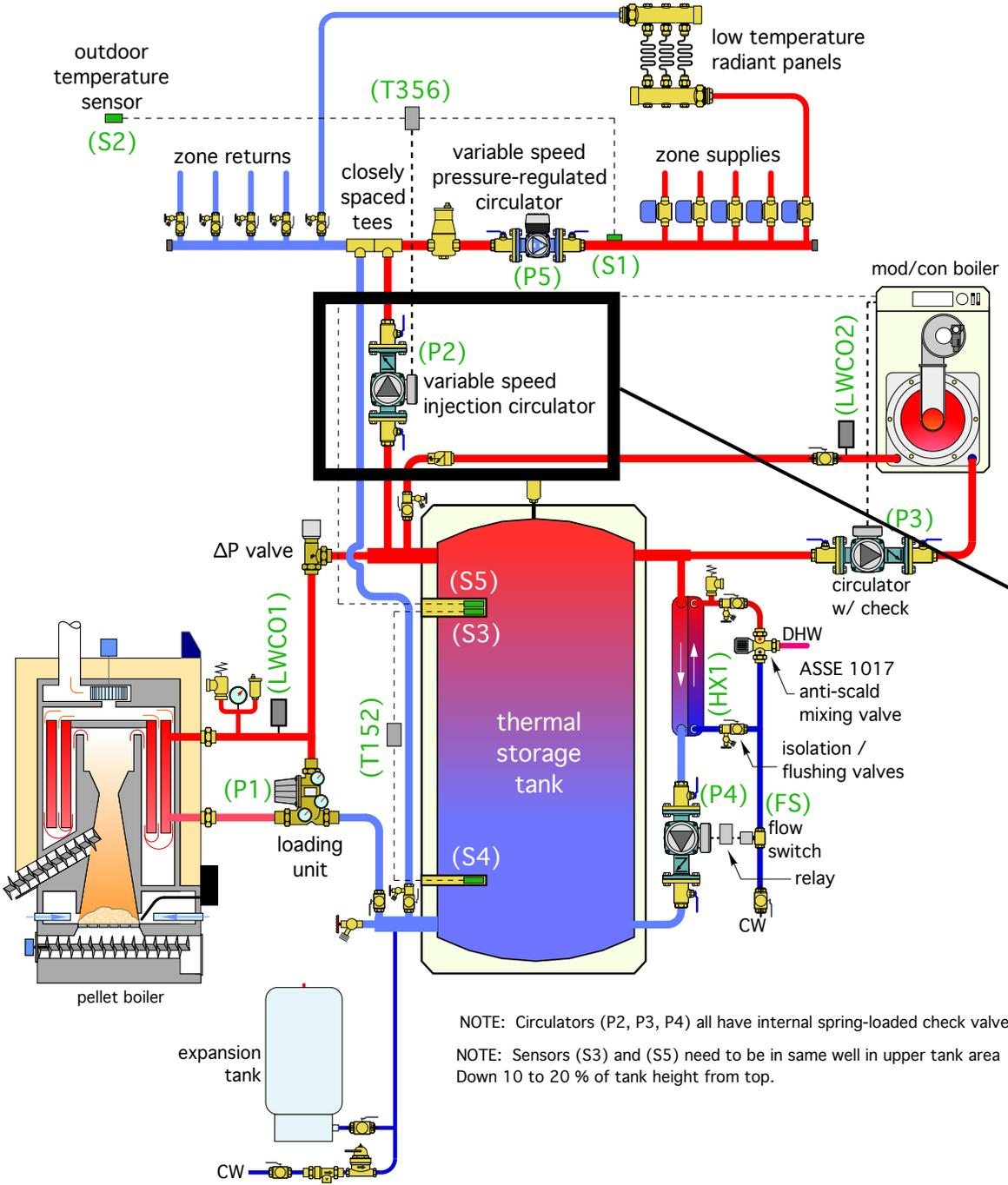
NOTE: Circulators (P2, P3, P4) all have internal spring-loaded check valves
