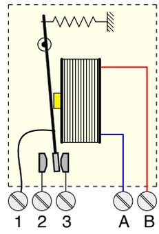
**Energized mode:** Voltage is applied to coil (terminals A and B). Pendulum pivots toward coil. The common contact touches the normally open contact. Current can flow from terminal 1 to terminal 3.
