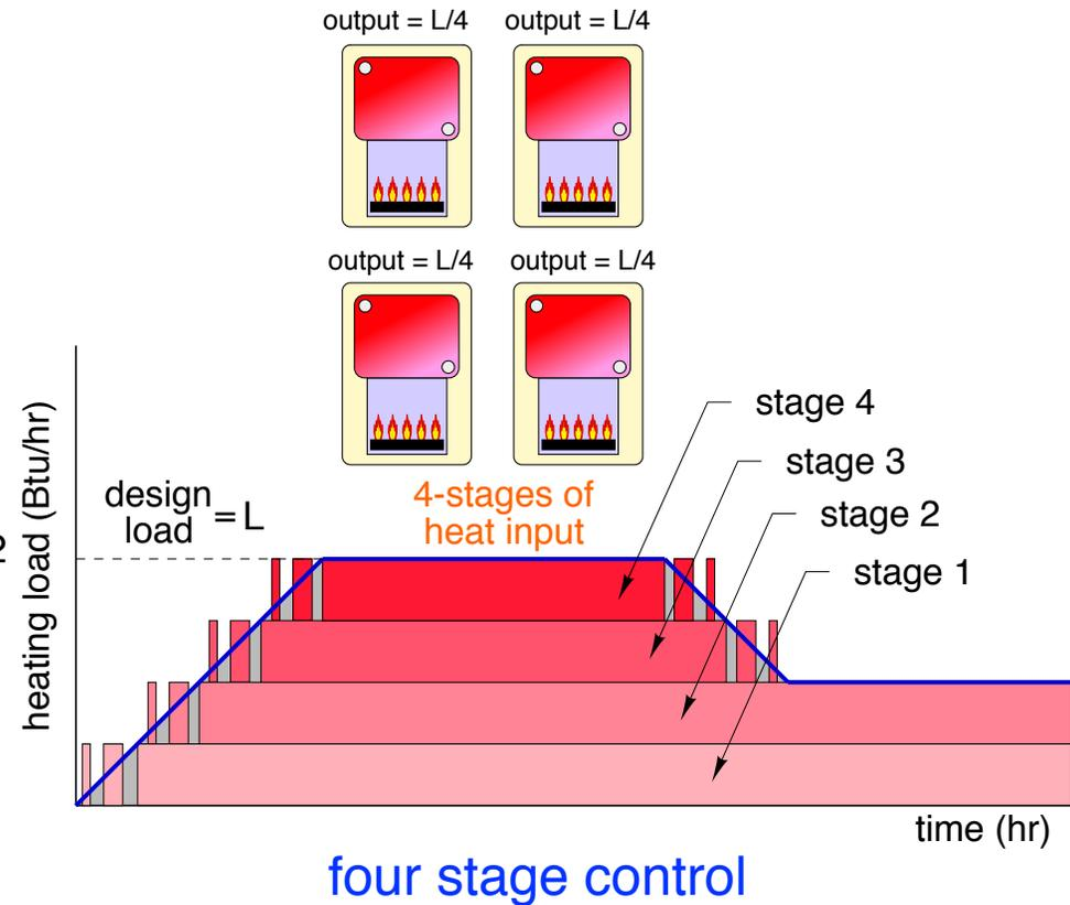
In theory, the greater the number of stages, the better the ability to match heat output to load. However, the cost of the installation also increases with increasing number of stages.
