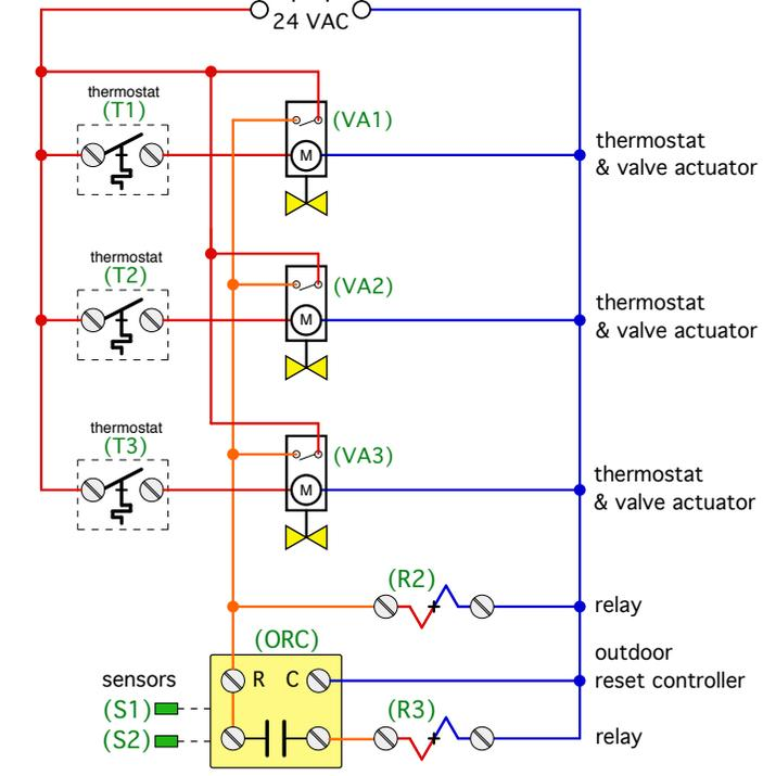
**Design tip: Always make sure that all electrically powered components have the same designator in the piping schematic and ladder diagram.**
