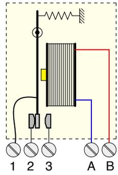
**"Normal" mode:** No voltage is applied to coil (terminals A and B). Spring holds pendulum so the common contact touches the normally-closed contact. Current can flow from terminal 1 to terminal 2.
