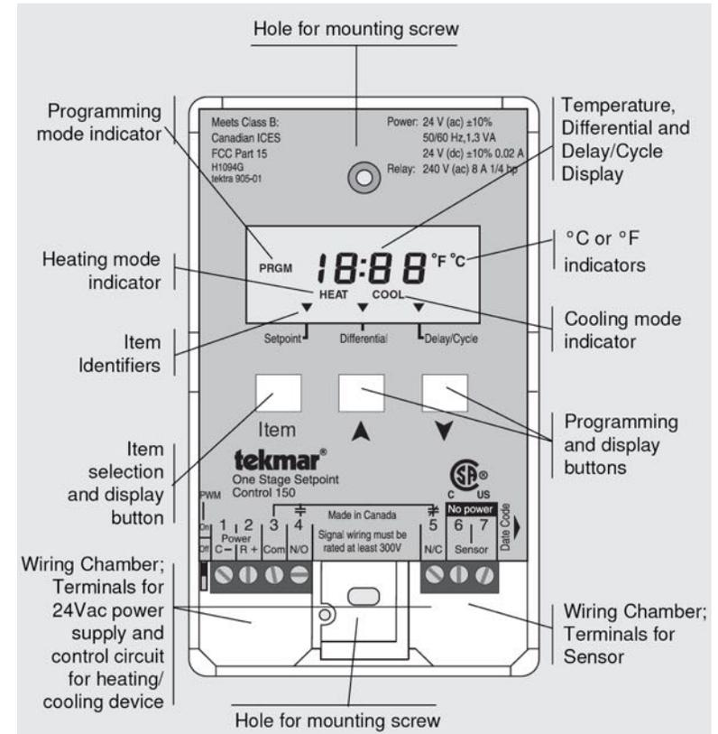
**Design tip: Always check max sensor wiring distance, and use 18 ga copper twisted pair or shielded cable when running long distances (minimizes electrical noise interference)**
