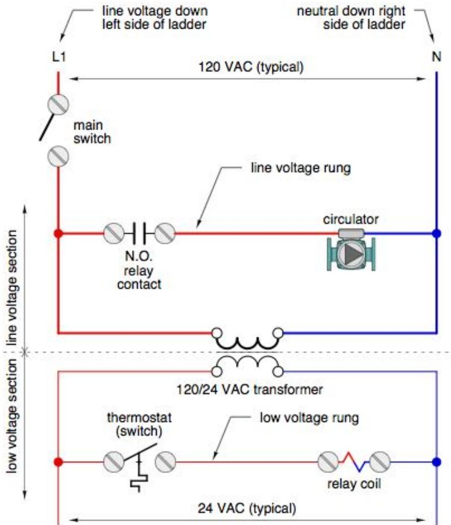
Two sections in a ladder diagram:
