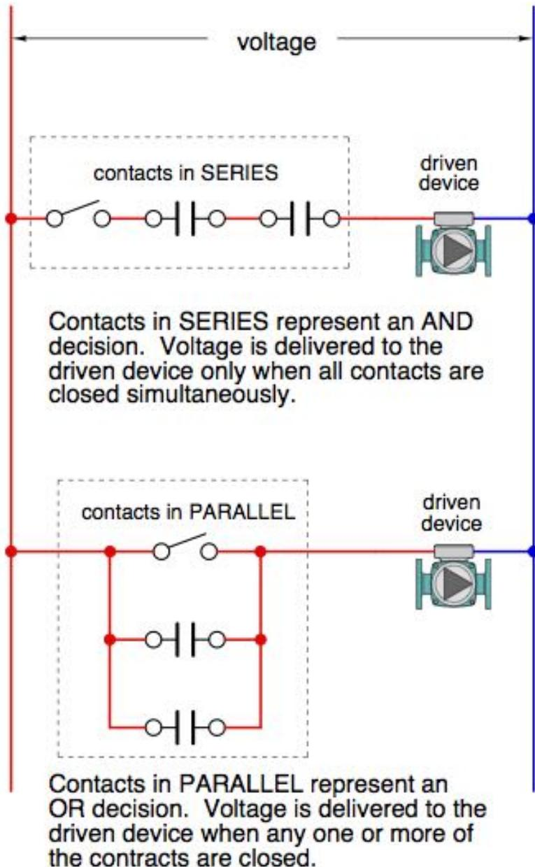
contacts in series represent an AND decision. All contacts must be closed simultaneously for a complete circuit.
