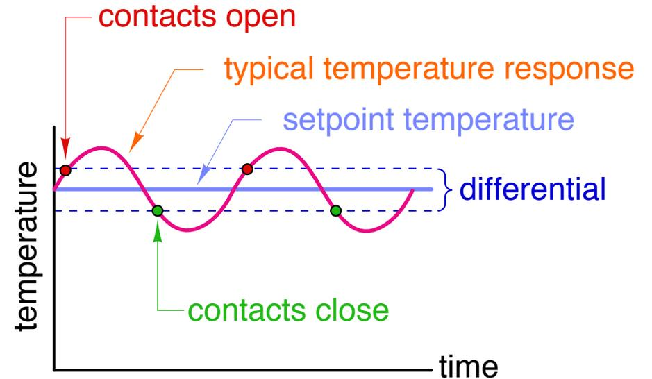
If the differential is too wide, the variable being controlled can drift far from the target.
