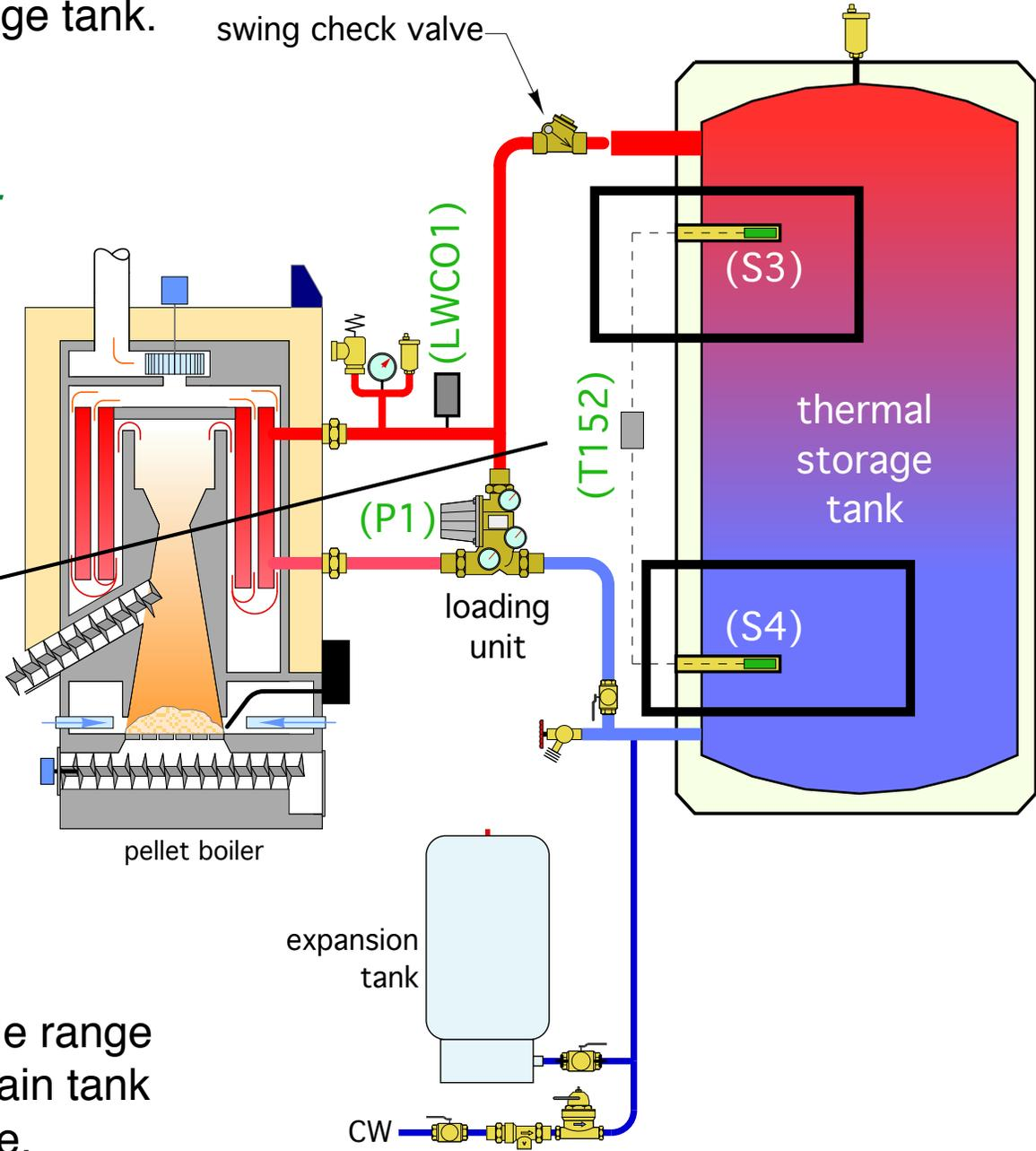
These temperature allow a relative wide range of tank temperature cycling, and maintain tank hot enough to provide DHW at any time.
