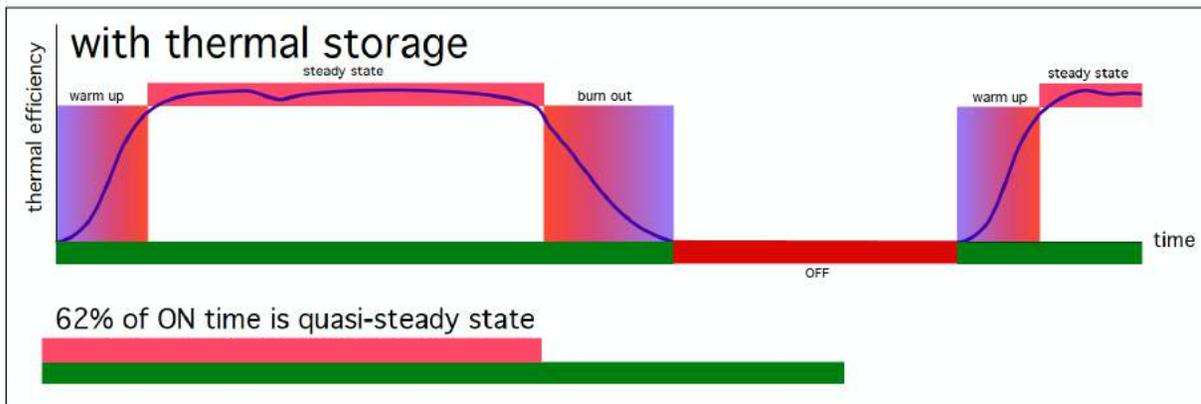
In most applications, pellet boilers require substantial thermal storage *(typically 2 gallons / 1000 Btu/hr boiler output)* to achieve these long operating cycles.
