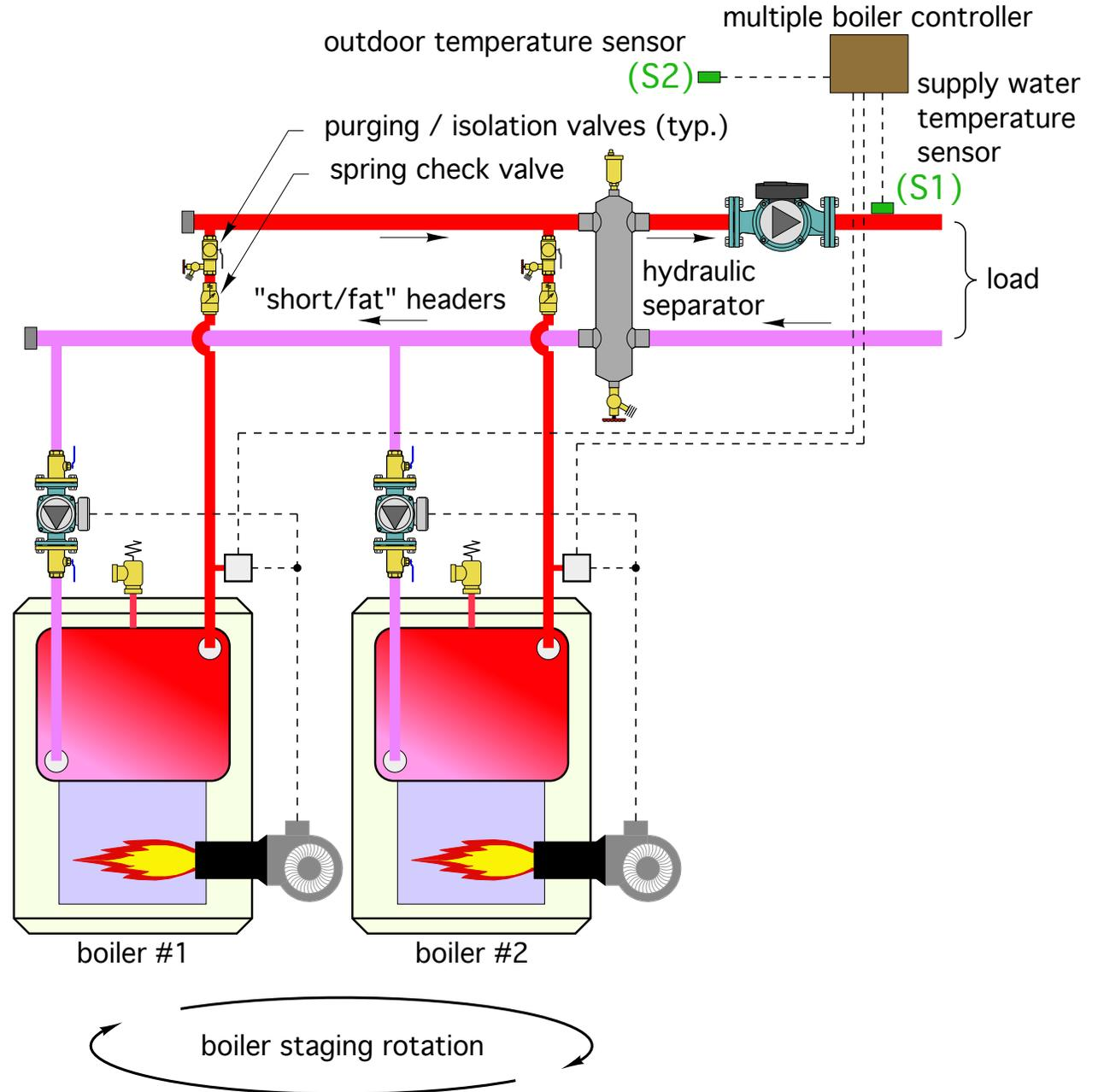
It's "intuitive" for designers to create systems where the biomass boiler is treated as a "fixed lead" stage, and the auxiliary boiler is the "lag" stage.
