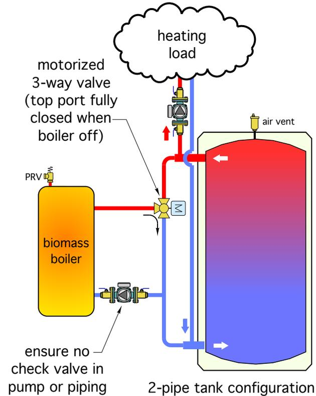
ensure no check valve in pump or piping
