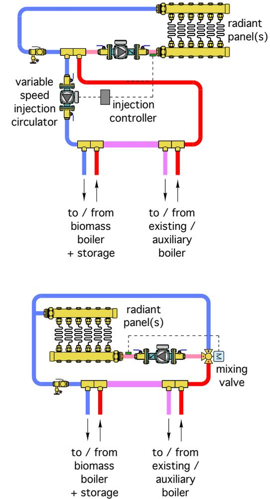
**If distribution system uses low water temperature (< 130 °F) don't forget to protect the aux boiler against sustained flue gas condensation**
