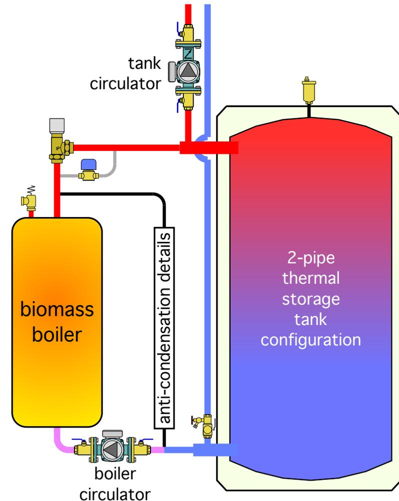
A typical pellet boiler is turned on and off based on temperatures in thermal storage. **(It operates independently of “calls” for heat from zone thermostats)**
