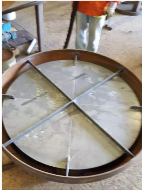
Baffle plate being welded into tank head & base shell at Troy Boiler Works
