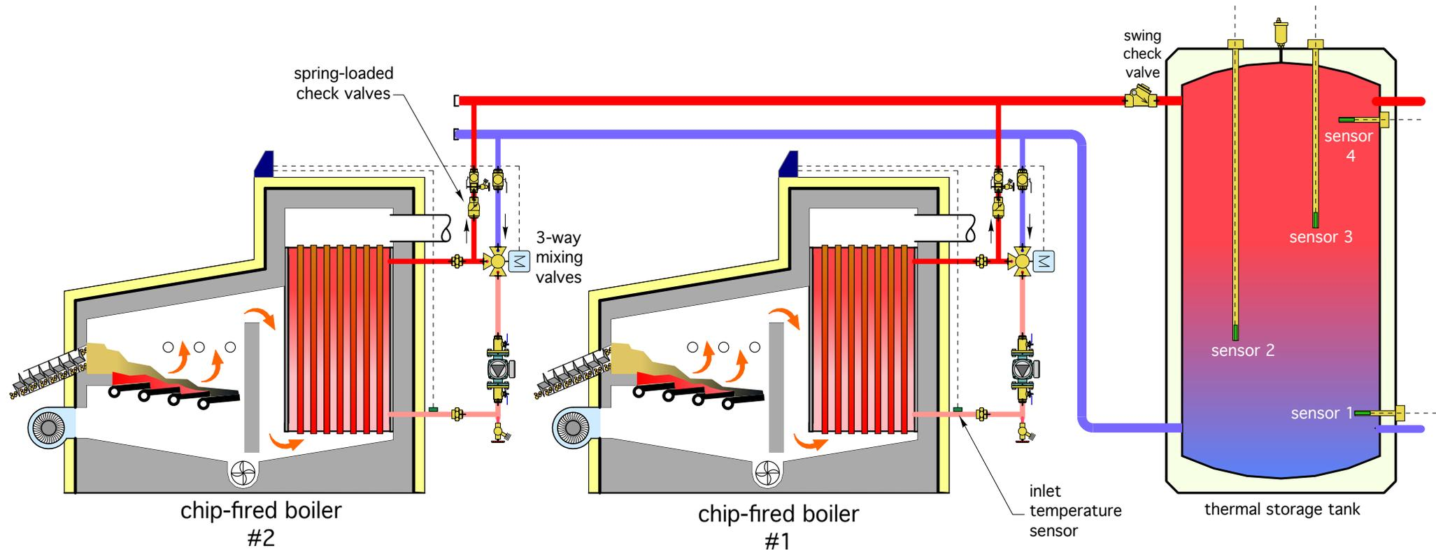
Firing order of boilers is periodically changes to help equalize boiler operating hours.
