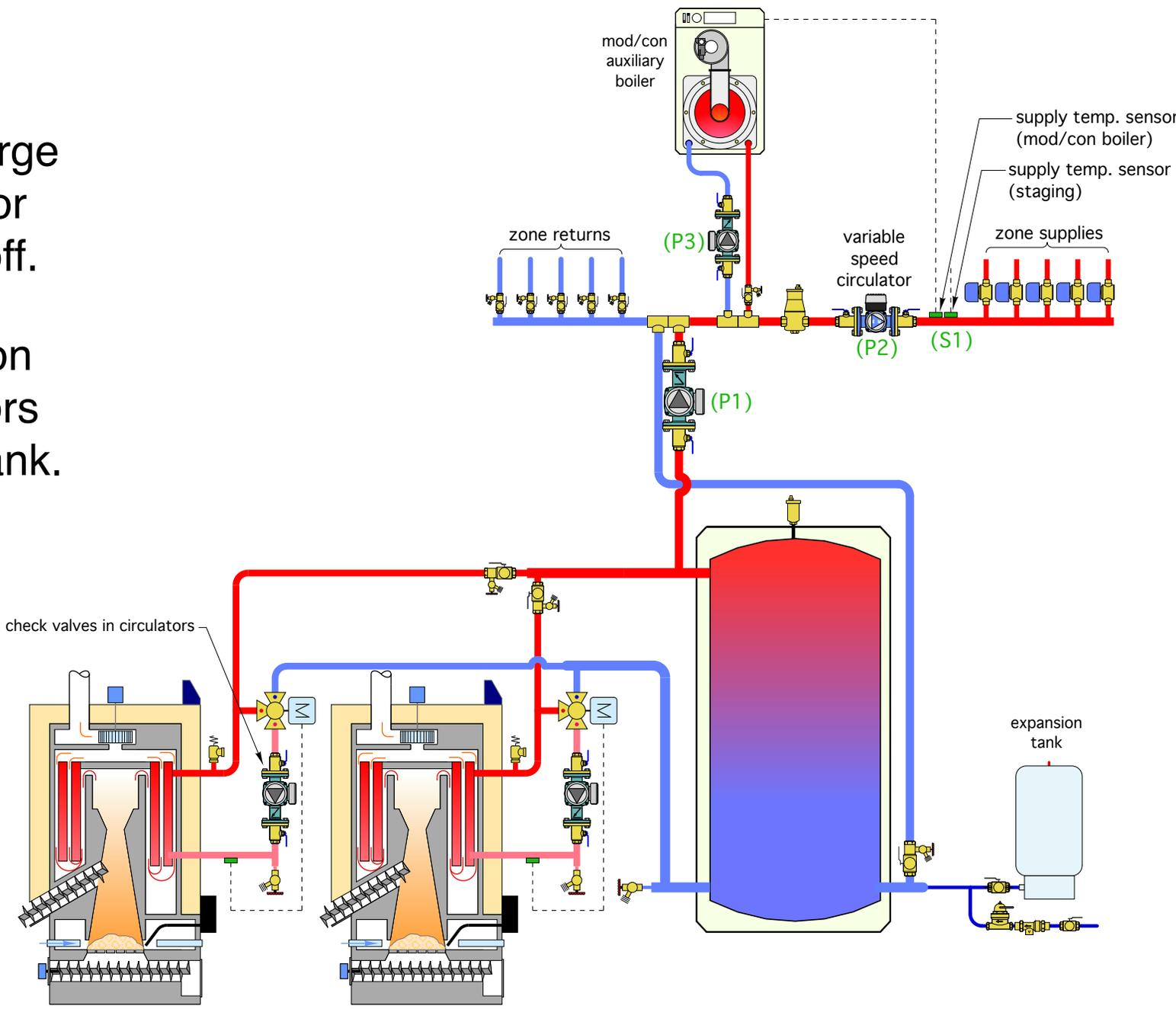
individual 3-way motorized valves for anti-condensation protection
