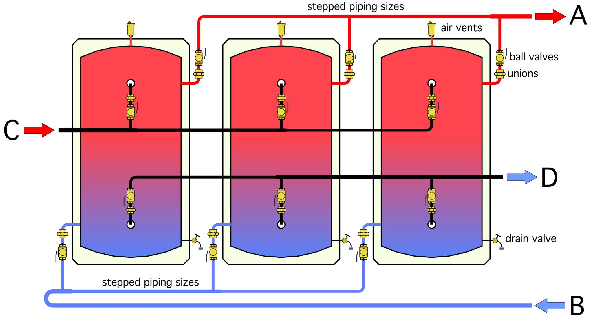
If using this piping be sure to plan for possibility of individual tank isolation and removal.
