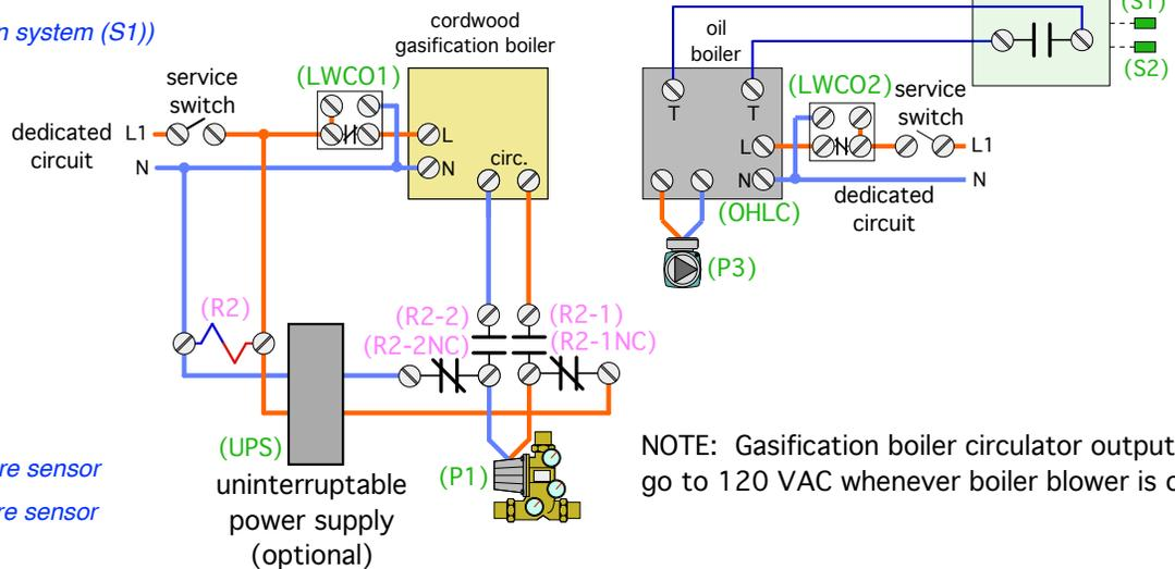
NOTE: Gasification boiler circulator output must go to 120 VAC whenever boiler blower is on
