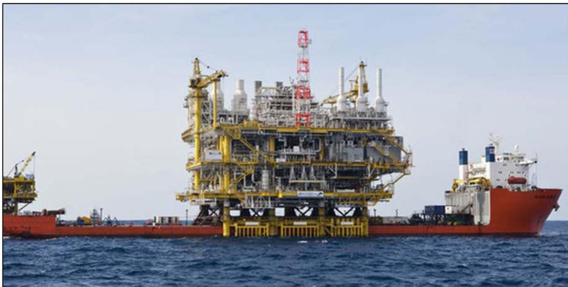
The Installation Contractor’s HLV will rendezvous with the HTV at the offshore site and lift directly off the HTV deck.
