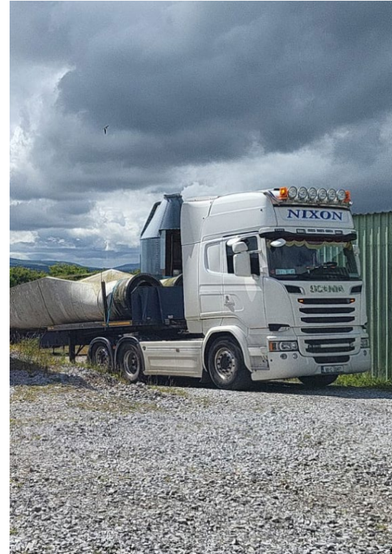
Decommissioned LM13.4 blade
