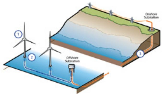
1. Offshore turbines capture the wind's energy and generate electricity.
