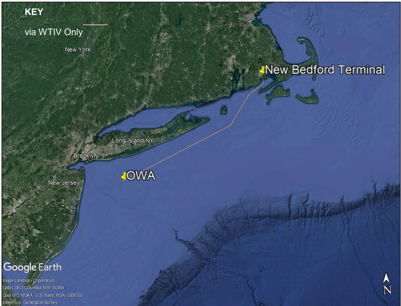
**Scenario 2.** WTIV and two jack-up feeder barges as seen in Figure 9: The feeder barges complete continuous round-trips from the New Bedford Terminal to the OWA, a steaming distance of approximately 222 km (120 nautical miles). On arrival at the OWA, the components are installed directly from the feeder barge by the WTIV, which stays on the project site at all times. Scenario parameters are based on the Vessel Study.
