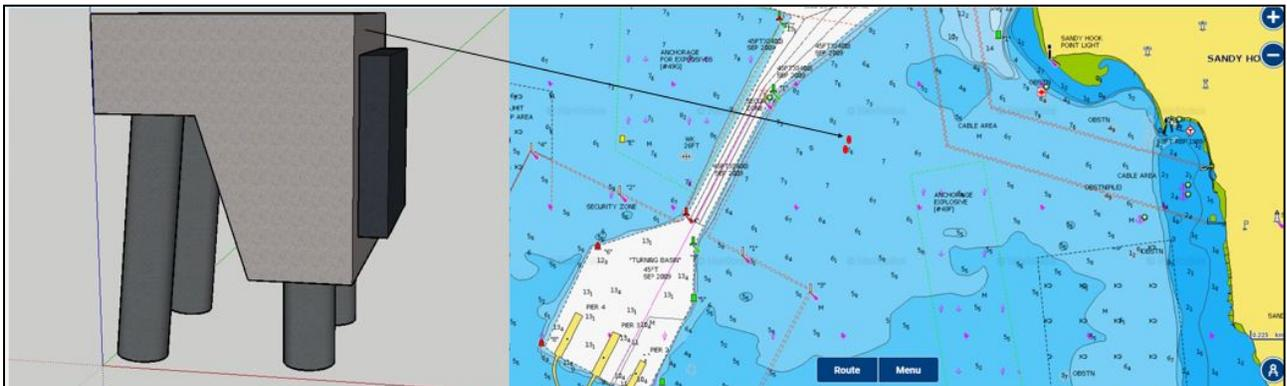
The mooring system consists of a mooring buoy connected to an anchor with a chain or combined wire and chain; the system occupies an area of approximately 22.7 hectares (56 acres). A mooring pennant on the chain beneath the buoy is recommended for ease of pick up and connection to the barge. The mooring system and various anchors alternatives are illustrated in the Figure 3.
