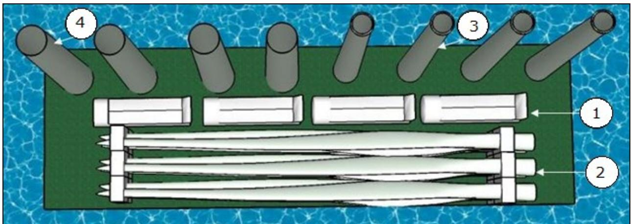
**Figure 21. Typical 400-Foot Barge Deck Layout for OSW Components**
