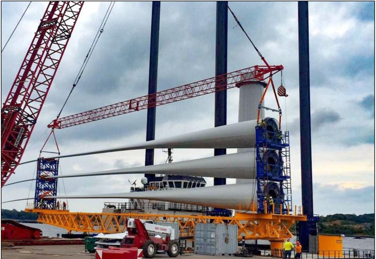
**Figure 6. WTIV Deck Loaded with OSW Components**
