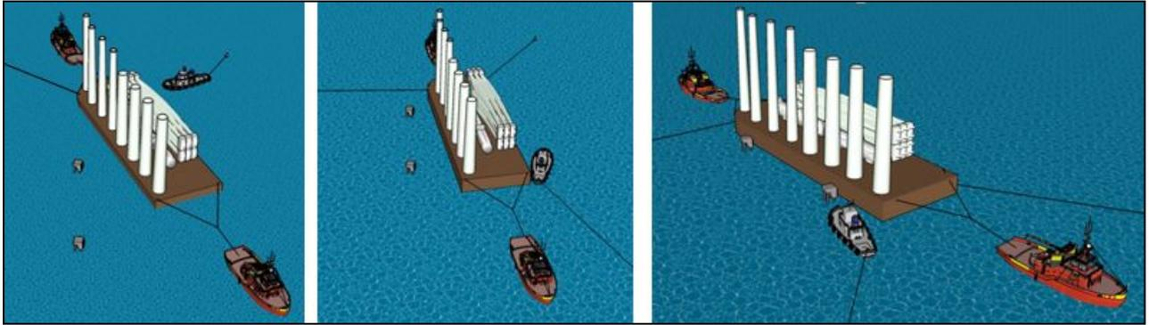
When the barge is moored and ready to transfer components, the WTIV will come in and jack-up next to the barge in order to lift the components from the barge to itself. The blades will be lifted on first, in sets of two or four, then the nacelles will be transferred, followed by the tower sections. Figure 5 and 6 show the component transfer process.
