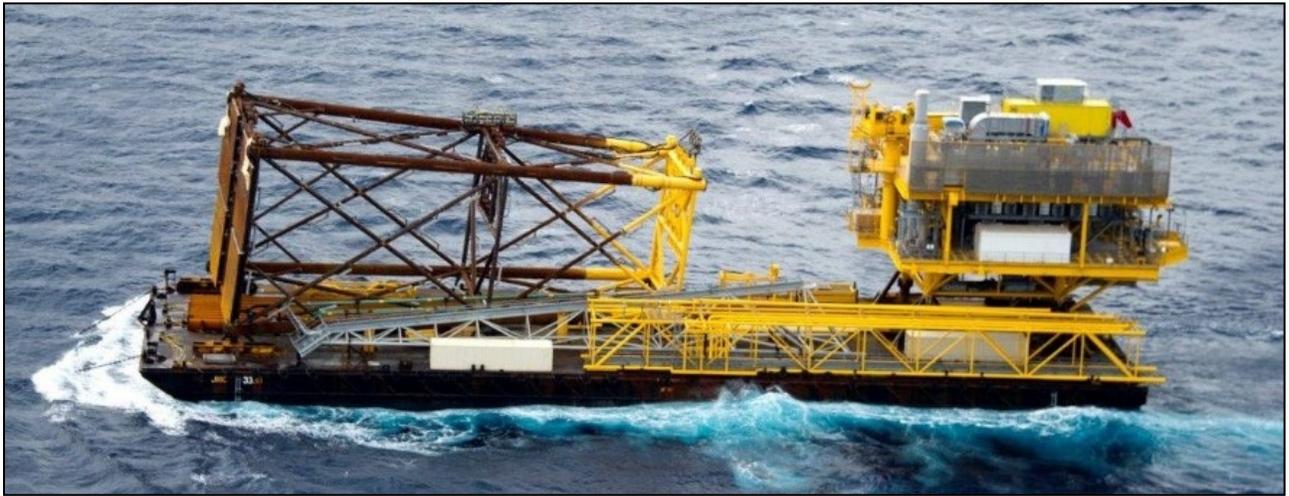
The 400-foot barge is based on the Cashman *Miss Hannah* vessel and has dimensions (l x b x d): 121.9 m x 36.6 m x 7.6 m (400 ft. x 120 ft. x 25 ft.) with deck capacity of 25 MT/m<sup>2</sup> (5,120 psf). The specification sheet for the *Miss Hannah* barge is included in the appendix. Figure 19 is a picture of the *Miss Hannah* barge.
