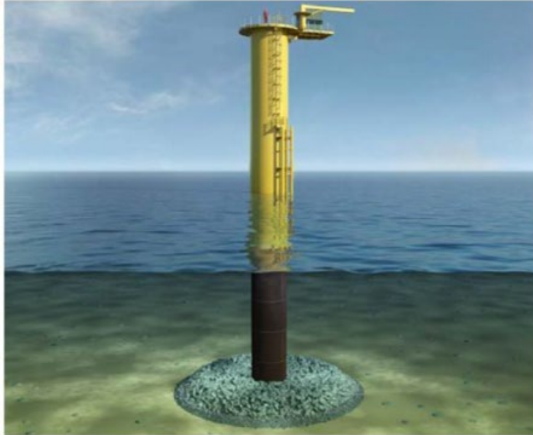
Figure 6.12: Typical Monopile Foundation with Transition Piece
