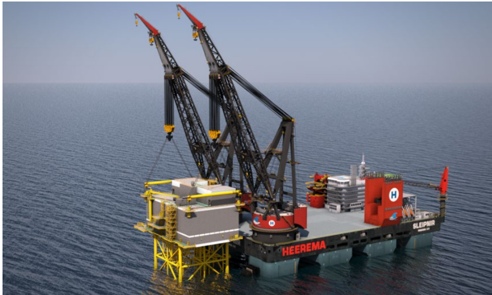
Figure 6.25: Rendering of HLV Used for Offshore Substation Installation
