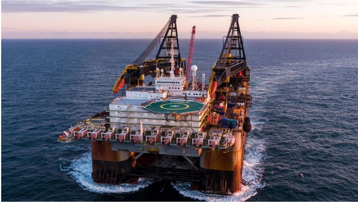
Figure 6.20: Semi-Submersible Vessel The Thialf
