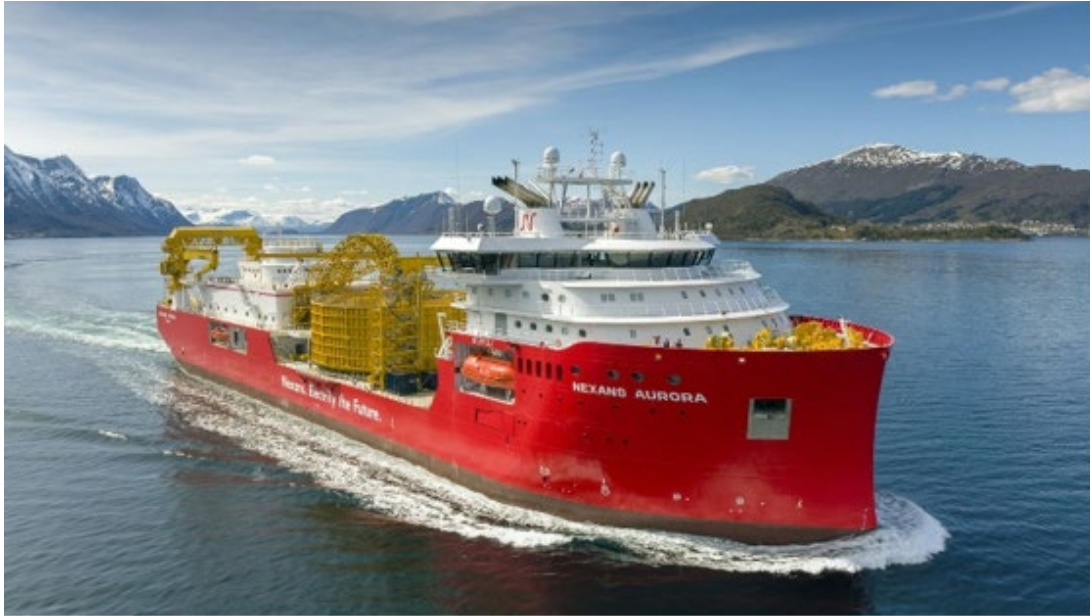
Figure 6.23: Typical CLV in Operation
