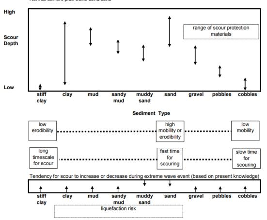
Conceptual model of the relative scour depth for different sediments in the marine environment Normal current plus wave conditions
