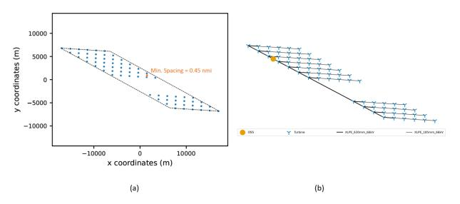
Figure 10. For Scenario 4 (a) optimized turbine layout (minimum turbine spacing specified) and (b) array cable configuration diagram
