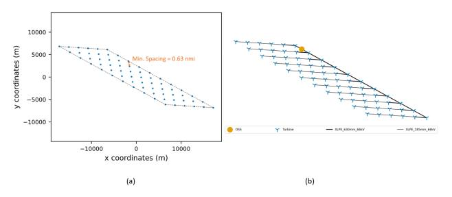
Figure 7. For Scenario 1 (a) optimized turbine layout (minimum turbine spacing specified) and (b) array cable configuration diagram
