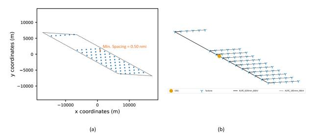
Figure 11. For Scenario 5 (a) optimized turbine layout (minimum turbine spacing specified) and (b) array cable configuration diagram
