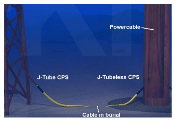
Articulated metal piping can be added to the cable to provide additional ballast and a higher level of cable protection using ductile or cast-iron half shells which link together. The application can be limited by water depths because of the considerable additional forces placed on the cable from the products weight which limits the deployable depths. However, they are feasible in the water depths found across the pilot project sites.
