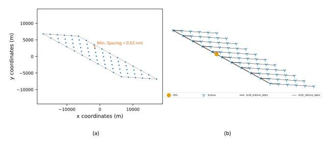
Note: Array cables are connected in series with a minimum separation distance of 65.6 ft (20 m). This distance is below the scale of Figures 6 - 12.
