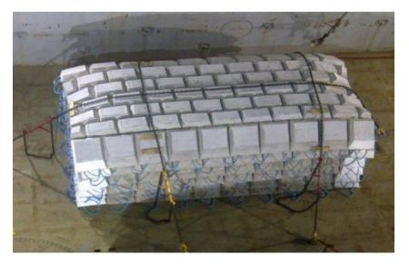
Rock bags come in differing weights and sizes. The advantage of using poly mesh bags allows the bag to be precision-deployed and, if needed, can be recovered later. These can be used to fill in seabed scour around OWF foundations or as cable protection as an alternative to concrete mattresses.
