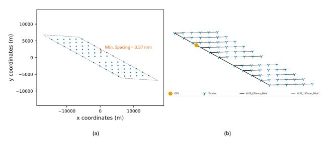
Figure 9. For Scenario 3 (a) optimized turbine layout (minimum turbine spacing specified) and (b) array cable configuration diagram
