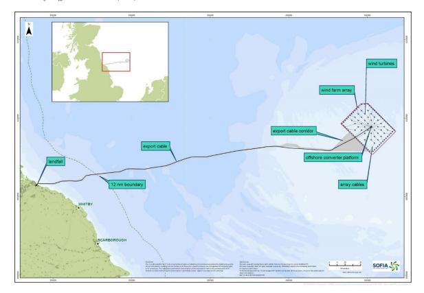
Minimizing north-south cable crossings was prioritized over maximizing the number of turbines per string based on the electrical current rating of the array cables. For the largest diameter array cable, these limits correspond to maximum of seven and five turbines per string for the 12 MW and 15 MW turbine ratings, respectively.
