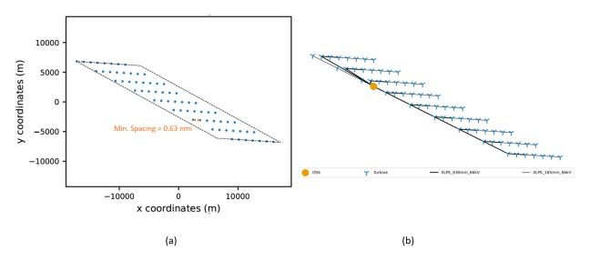
Figure 8. For Scenario 2 (a) optimized turbine layout (minimum turbine spacing specified) and (b) array cable configuration diagram
