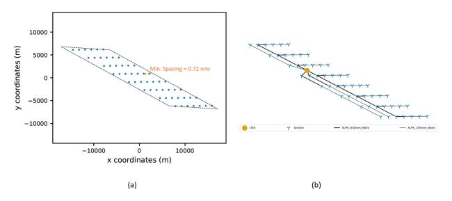
Figure 12. For Scenario 6 (a) optimized turbine layout (minimum turbine spacing specified) and (b) array cable configuration diagram
