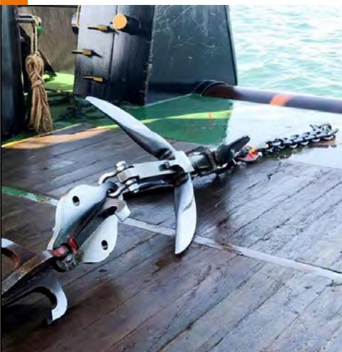
**Figure 22. Grapnels Containing Wire Rope Recovered to Deck**
