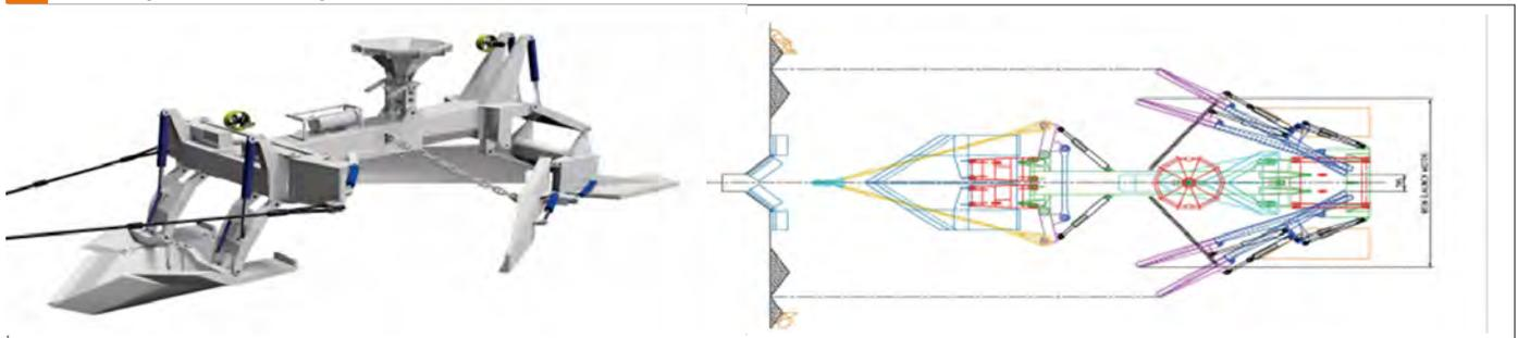
**Figure 66. Multimode Pre-lay Plow in Trenching Configuration**
