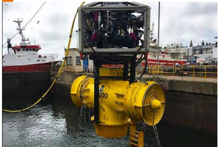
Figure 64. Sea Axe MFE, Maximum Flow Rate 5,600 L/second and Velocity 6.5 m/second (Courtesy, The JBS Group).
