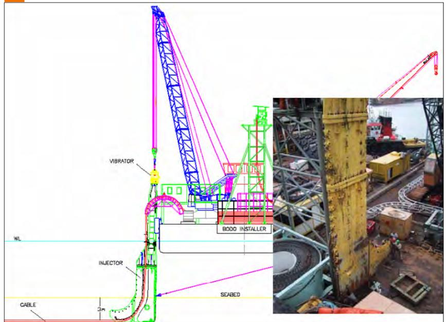
Figure 57. Vertical Injector Tool Schematic and Images (Courtesy, TenneT/Nordlink).
