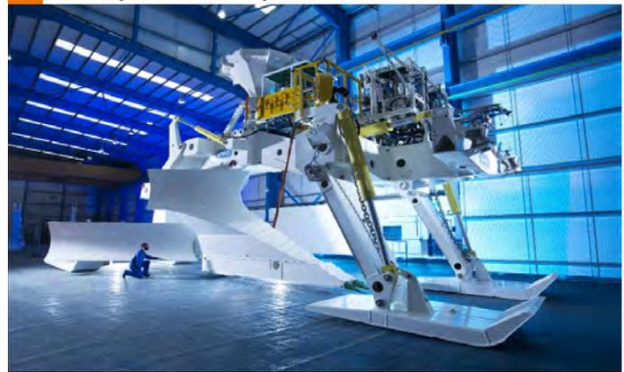
**Figure 68. Multifunction Pre-lay and Backfill Plow**
