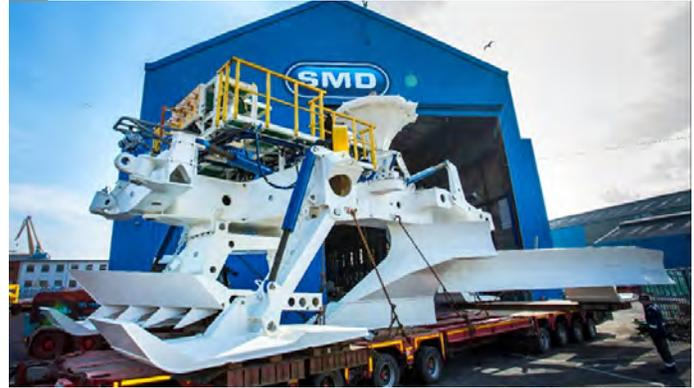
**Figure 67. Multimode Pre-lay Plow in Trenching Configuration**
