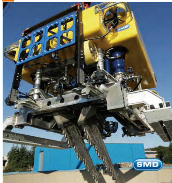
as fiber optics for video and data transmission. ROVs come in all shapes and sizes, from small observation class vehicles up to large, powerful work class vehicles. This section concentrates on the latter as work class vehicles are required to meet cable burial demands.
