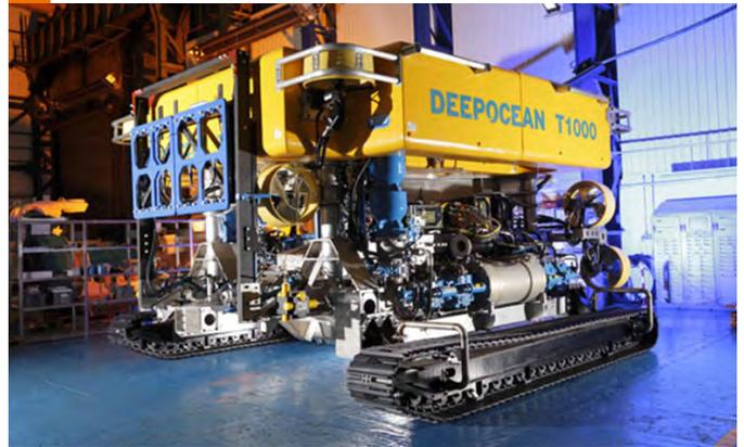
Figure 60. Trenching ROV in Free-Flying Mode Showing Jetting Tool
