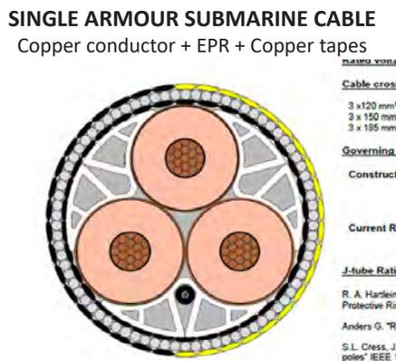
Figure 14. Components of Typical HVAC Export Cable
