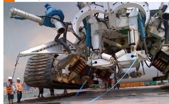
Figure 54. DeepOcean T3200 Mobilized onto the Havila Phoenix
