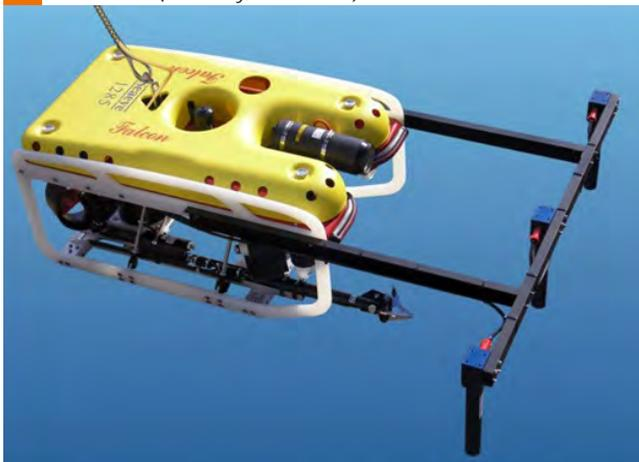
**Figure 85. Pangeo Sub-bottom Imager Mounted on a Work Class ROV (Courtesy, Pangeo Subsea).**
