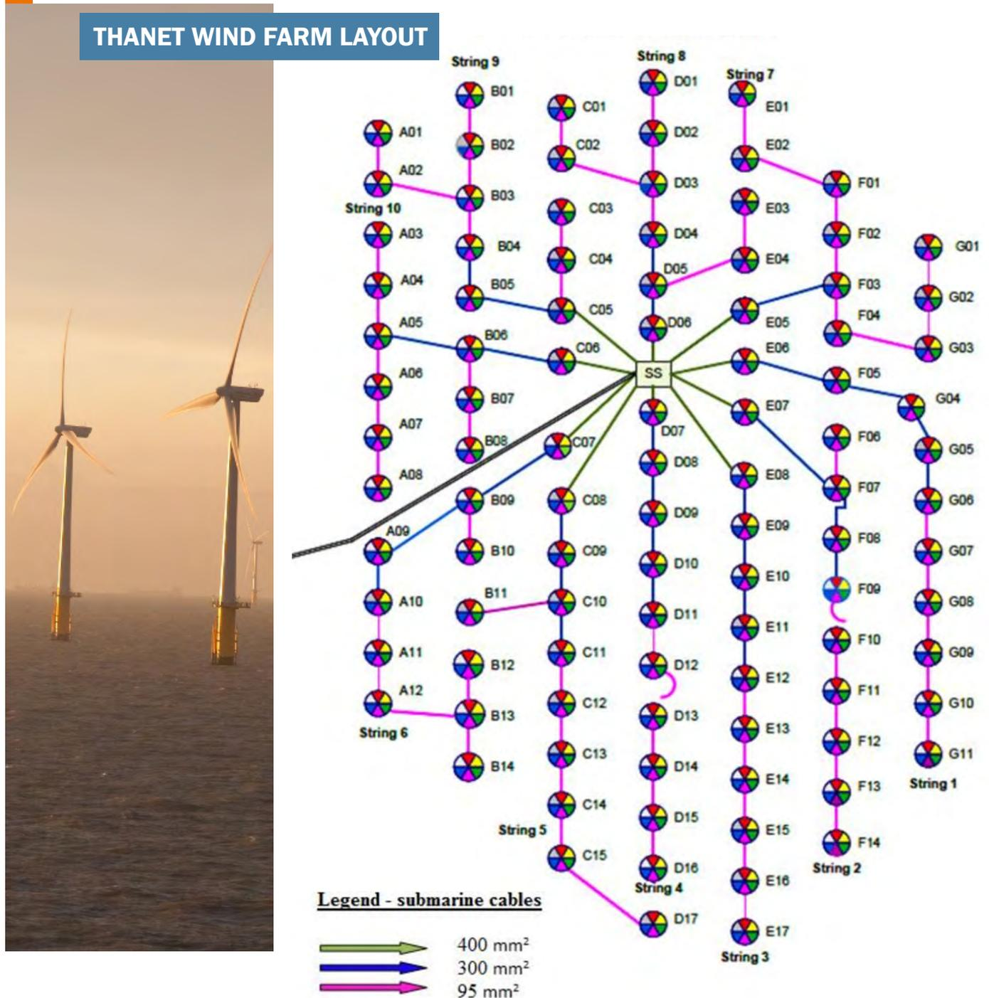
While the mechanics of laying array cables are mostly the same as for export cables, in practice, there are key differences. Array cables can be delivered in a variety of ways as they must fit the containment areas on the vessels that install them, including:
