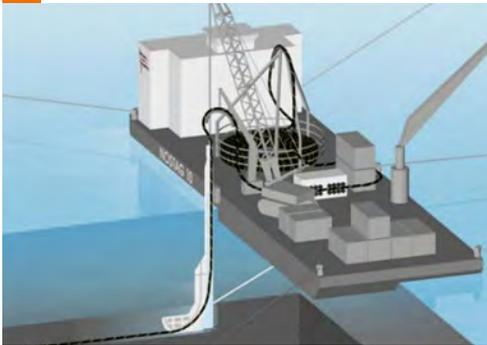
Figure 56. Vertical Injector Tool Schematic and View on Deck (for scale) (Courtesy, Burbo Bank Wind Farm).
