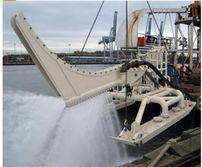
Figure 47. Large Jetting Sled (BSS-II) Suspended from a Crane During Launch (Courtesy, Boskalis). This sled can bury cable 25 ft (8.0 m) and also has a rock cutting tool capability.
