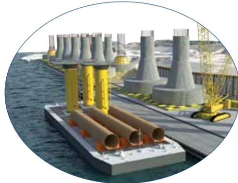
Some manufactured components will be floated down the Hudson River to a staging facility for final assembly before installation
