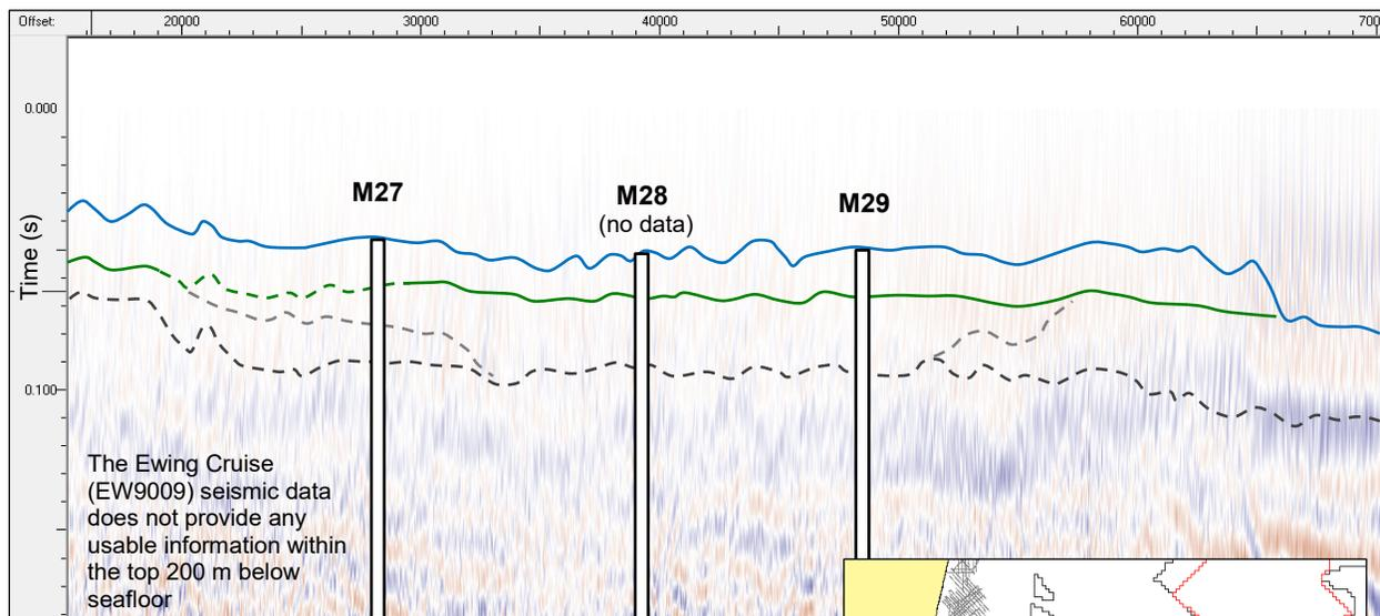
The top image reproduces seismic data acquired during the 1995 Oceanus cruise OC270 with a 48 channel, 600 m streamer and single 90 cui airgun. The majority of the data collected during that cruise was acquired east of the Hudson South site (Figure 4). Near seafloor resolution is not as good as that of the 1998 RV
