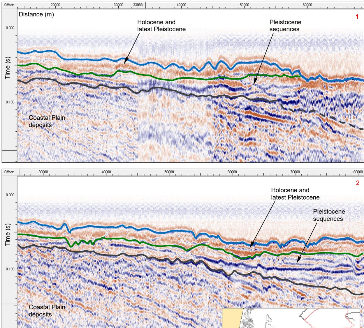
The above images reproduce further data acquired with the LDEO Portable HiRes Multi-Channel Seismic system during the 1998 RV Cape Hatteras cruise. The vertical extent of the images, from seafloor to the base of the images (140 ms), is approximately 120 m (410 ft).
