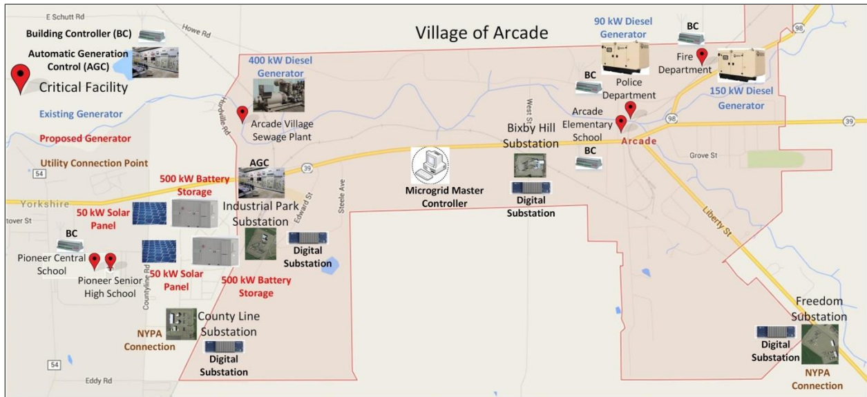
Figure 35. Network Equipment simplified layout diagram
