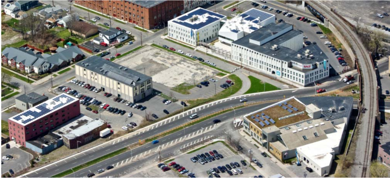
Figure 1.3 — Three adaptive reuse projects in the northeast corner of the Near Westside include a total of 138kW of existing solar photovoltaic generation that was included in the design of the envisioned microgrid: 1) WCNY, top (95 kW); 2) Lincoln Supply, left (31 kW); and 3) King+King, right (12 kW).
