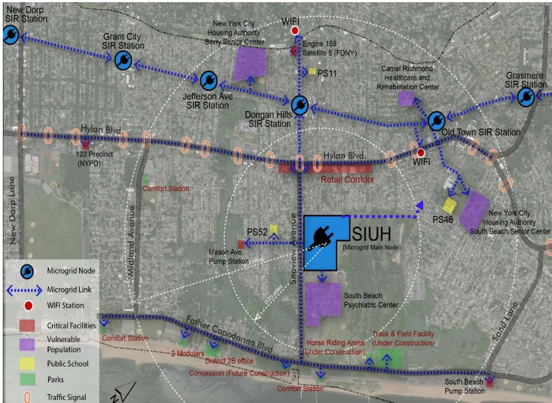
**Figure 1 – Potential Microgrid Participant Layout**
