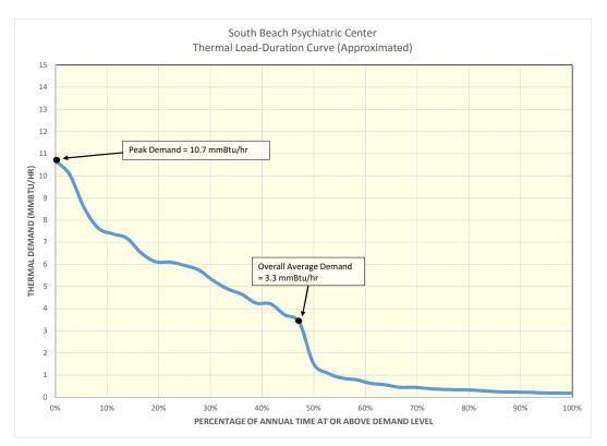
EXHIBIT 2.2.6 – APPROXIMATED SBPC THERMAL (HOT WATER) LOAD-DURATION CURVE
