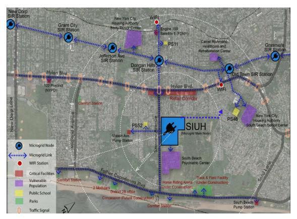
Figure 1 – Potential Microgrid Participant Layout
