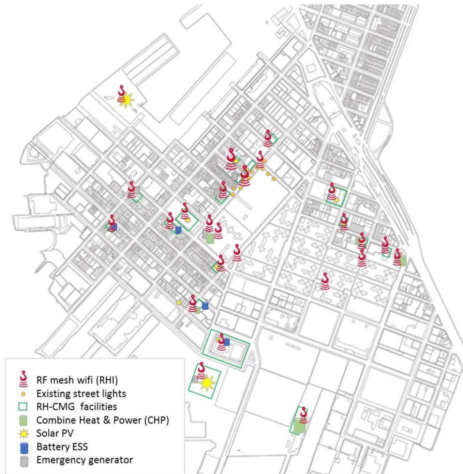
Figure 9: RH-CMG Communications Nodes – RHI RF Mesh
