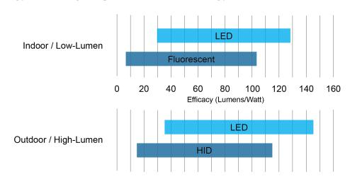
When replacing fluorescent or HID fixtures with LEDs, if the efficacy of the existing fixtures is unknown, then a wattage reduction of no more than 1/3 should be assumed.
