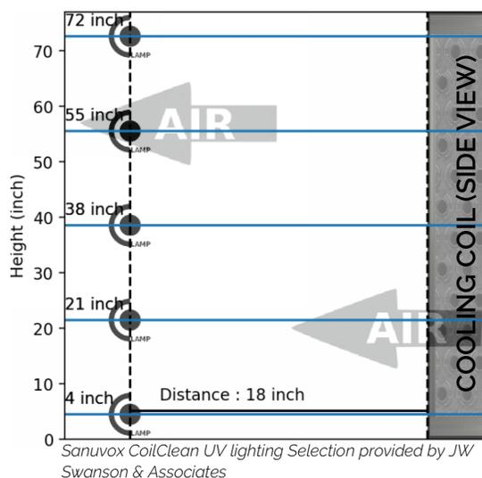
The graphs below shows the surface irradiation intensity across the coil's cross section for a 5-row, 10-lamp configuration located 18 inches away from the cooling coil. The average irradiation intensity for this configuration is 1,741  $\mu\text{W}/\text{cm}^2$ , which is enough to sufficiently kill all microorganisms on the surface of the cooling coil.
