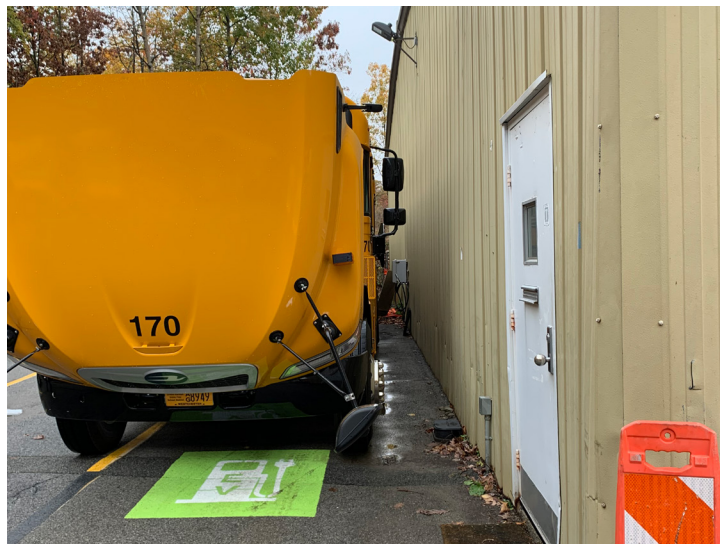
Level 2 chargers can be wall mounted to minimize footprint. An example installed in Croton-Harmon UFSD is mounted in the garage with a cut-through so buses can be charged inside and outside the maintenance garage.
