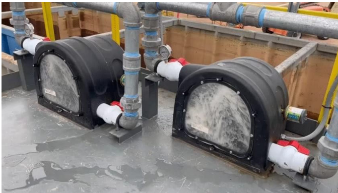
Water drives a pair of turbines at the Starr County test site. (Sage Geosystems)
