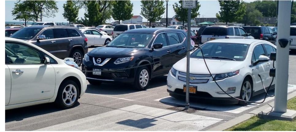
EVs have a portable charging cord that plugs into a 110V outlet and a site could provide only outlets for use by these portable cords as a very low cost option. However, EV charging outlets must be on a dedicated circuit and three-prong outlets will experience wear from everyday use (the EV connector was specifically designed for this).
