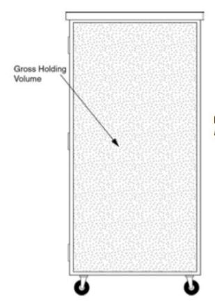
**Equation 1:** Interior Volume = Interior Height x Interior Width x Interior Depth
