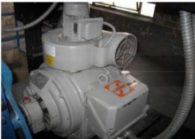
Figure 3: AC motor with VVVF control
