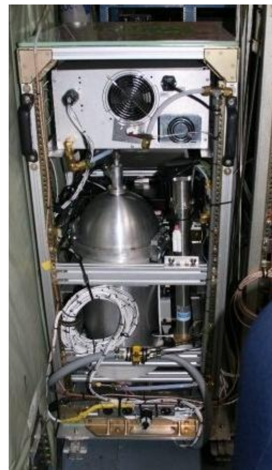
FIG10: HDDMA located in 19 inch rack in C-130 aircraft to measure particle size distribution in upper atmosphere
